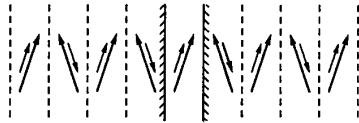
Fig. 1. Reference direction of images and the respective currents for a branch between two parallel metal plates.
