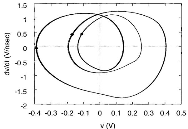
Fig. 12. Three-cycle oscillation phase space. The injection signal is as in Fig. 11. The markers indicate the points of the Poincaré sectioning. The thickness of the lines indicates that the system has not completely settled, which could be eliminated with significantly longer execution times.
