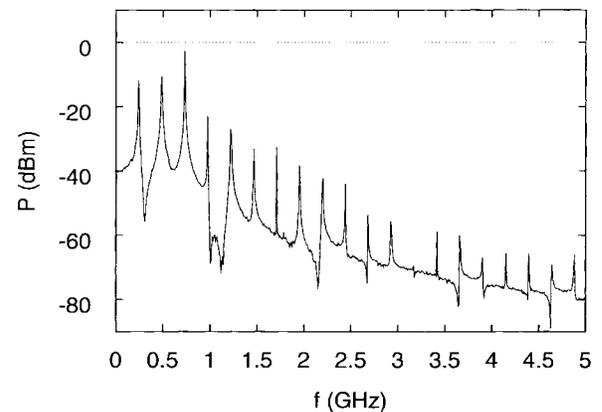
Fig. 13. Three-cycle oscillation frequency domain. The parameters are again as in Fig. 11. The noise floor is roughly the same as Fig. 10. The power in the fundamental frequency is much less than seen in Fig. 10.
