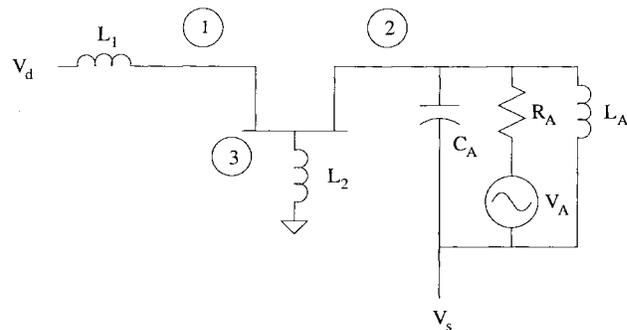
Fig. 1. Source–load oscillator topology with the circuit nodes numbered. Node 2 is the source of the transistor, which is coupled to a tank circuit and drive voltage.
