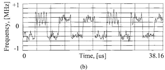
Fig. 15. (a) Received and frequency shift-keying (FSK) demodulated 50-kHz signal for a receiver located at  $0^\circ$ . (b) Received and FSK demodulated 150-kHz signal for a receiver located at  $20^\circ$ . The signals are demodulated using a vector signal analyzer.
