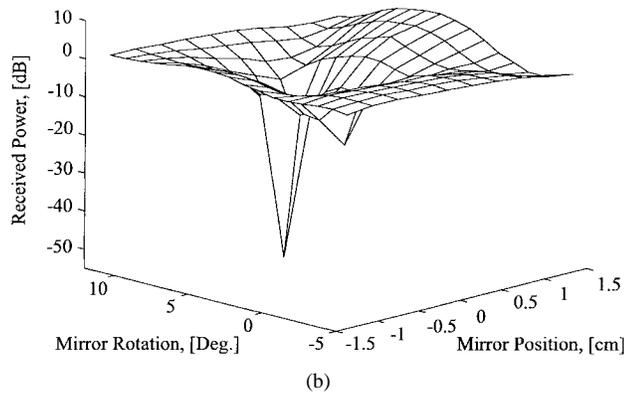
Fig. 12. Measured maximum multipath fading nulls of a 10.1-GHz carrier signal. The received power is normalized to through measurements without the mirror inserted. (a) With and (b) without the 24-element lens amplifier array inserted. Notice the different vertical scales.
