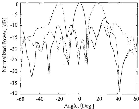
Fig. 13. Beamscanning in  $E$ -plane at 10.1 GHz for the 24-element lens amplifier array in receive mode. Receive horn at  $(-)$   $0^\circ$ ,  $(- -)$   $-20^\circ$ , and  $(\cdot \cdot \cdot)$   $20^\circ$  locations are shown. The normalizing power levels of the main lobes are within 2 dB.
