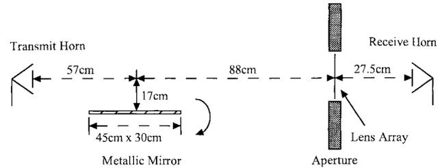
Fig. 11. Test setup for the multipath experiment. A  $45 \text{ cm} \times 30 \text{ cm}$  metallic mirror located parallel to the optical axis in front of the 24-element lens amplifier is translated in 3-mm steps from the axis. For each step, the mirror was rotated through a set of angles.
