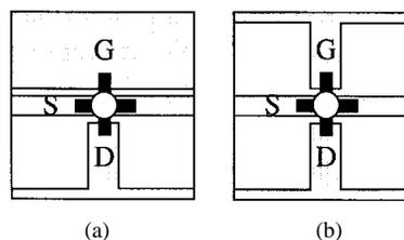
Fig. 14. Unit cell of a grid oscillator with (a) slot/dipole radiating elements and (b) dipole radiating elements. Both cells are 6-mm square and are loaded with HP-Avantek ATF-26884 MESFET's. The grids are printed on a 0.5-mm substrate (Duroid 5880,  $\epsilon_r = 2.2$ ) and placed on a second 5-mm layer (Duroid 6010.8,  $\epsilon_r = 10.8$ ) which is metallized on the back.
