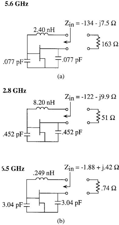
Fig. 10. Negative-resistance model for the grids associated with (a) Fig. 5(a) and (b) Fig. 5(b).
