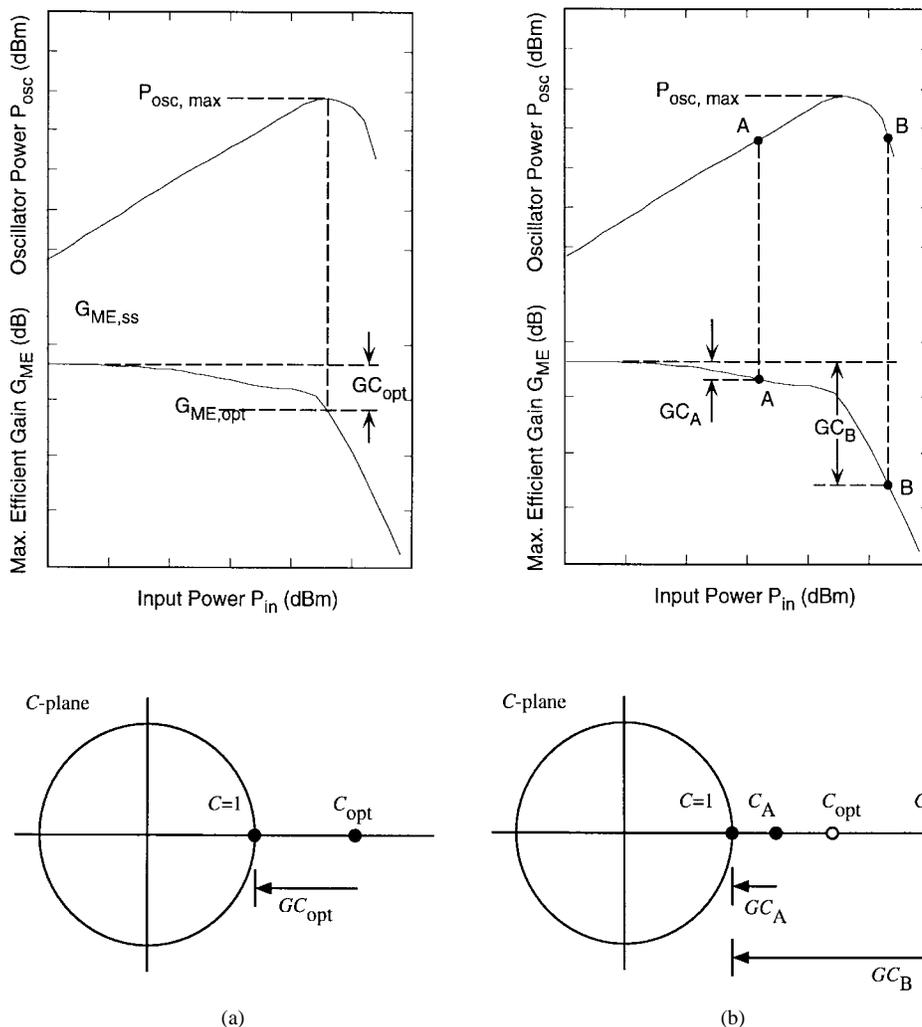
Fig. 12. Transistor saturation characteristics and circular-function plane for (a) the optimal operating point, and (b) two suboptimal operating points.  $P_{in}$  is the input power to the transistor, as indicated in Fig. 2(b), and  $P_{osc} = P_{out} - P_{in}$  is the radiated power.
