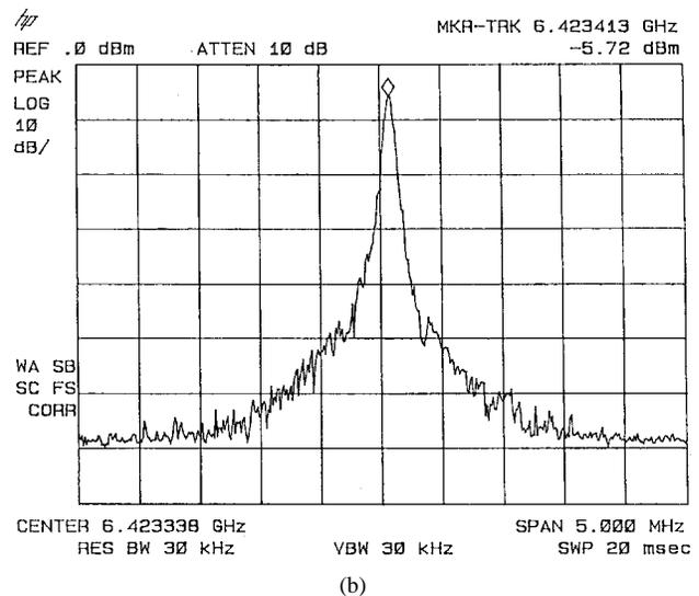
Fig. 6. Measured oscillation modes for a  $6 \times 6$  grid backed by a high-permittivity substrate and mirror. (a)  $2.7$  GHz. (b)  $6.4$  GHz. Each mode was obtained separately at different dc bias currents:  $5$  mA/device for (a) and  $12$  mA/device for (b).
