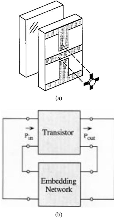
Fig. 2. (a) Unit cell of a grid oscillator with the transistor and passive grid separated. (b) Feedback-oscillator model consisting of the embedding network and the transistor model.  $P_{in}$  and  $P_{out}$  represent the input and output power of the transistor, respectively. The power dissipated in the embedding network  $P_{out} - P_{in}$  is the actual power radiated by the grid oscillator.
