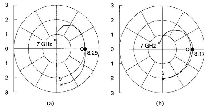
Fig. 15.  $C$ -functions for the (a) slot/dipole- and (b) dipole-grid oscillators. The shaded symbols represent the  $C$ -functions of the grids, and the open symbols represent the  $C$ -functions of the theoretical optimum networks.
