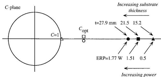
Fig. 13. Operating points corresponding to three different substrate thicknesses for a C-band pHEMT grid oscillator. The shaded symbols represent the  $C$ -functions of the grids, and the open symbols represent the  $C$ -functions of the theoretical optimum networks. The measured ERP is also shown.
