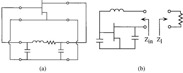
Fig. 9. (a) Transistor connected to the equivalent  $\Pi$  network. (b) Negative-resistance model of the grid oscillator.
