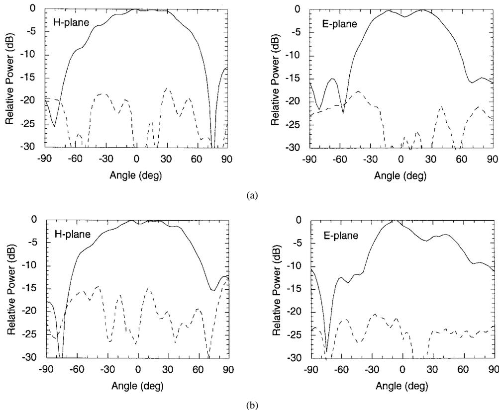
Fig. 16. Measured  $H$ - and  $E$ -plane patterns of the (a) slot/dipole- and (b) dipole-grid oscillators of Fig. 14. Solid lines represent the copolarization and dashed lines represent the cross polarization.
