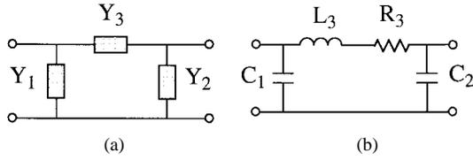
Fig. 8. (a) General lumped equivalent circuit for a two-port network, where  $Y_1 = Y_{11} + Y_{12}$ ,  $Y_2 = Y_{22} + Y_{12}$ , and  $Y_3 = -Y_{12}$ . (b) Typical form of the equivalent circuit for a grid.
