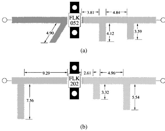
Fig. 1. Microstrip layout of: (a) the class-F amplifier using the FLK052 and (b) the class-E amplifier using the FLK202. The substrate is 0.508-mm-thick RT5880 Duroid ( $\epsilon_r = 2.2$ ). All dimensions are given in millimeters.
