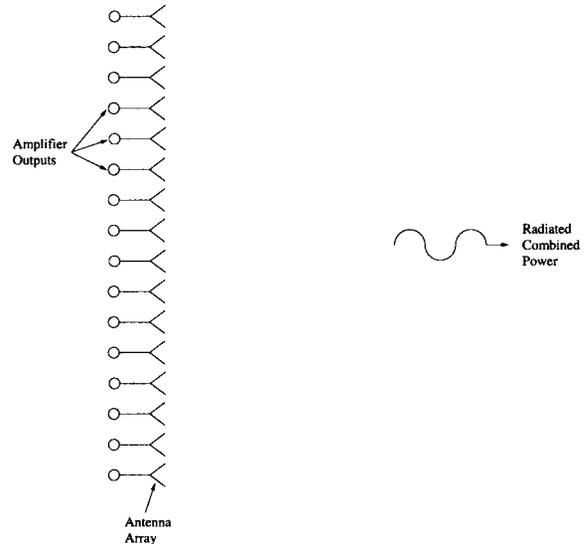
Fig. 5. Spatial power combiner. The output of an amplifier is connected to each circle.
