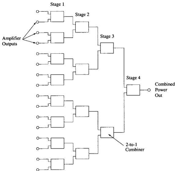
Fig. 4. A circuit corporate power combiner. The output of an amplifier is connected to each circle.
