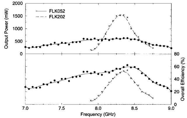
Fig. 2. Output power and overall efficiency versus frequency for the FLK052 class-F amplifier (solid line) and the FLK202 class-E amplifier (dashed line). The input power is 20 dBm for the FLK052 class-F amplifier and 26 dBm for the FLK202 class-E amplifier.  $V_{\text{DS}} = 7.0$  V and  $V_{\text{GS}} = -0.9$  V.
