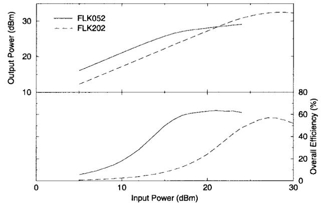
Fig. 3. Output power and overall efficiency versus input power for the FLK052 class-F amplifier (solid line) and the FLK202 class-E amplifier (dashed line). The frequency is 8.4 GHz for the FLK052 amplifier and 8.35 GHz for the FLK202 amplifier.  $V_{\text{DS}} = 7.0$  V and  $V_{\text{GS}} = -0.9$  V.
