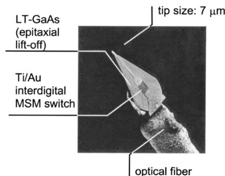
Fig. 1. Micromachined photoconductive probe with optical fiber.
