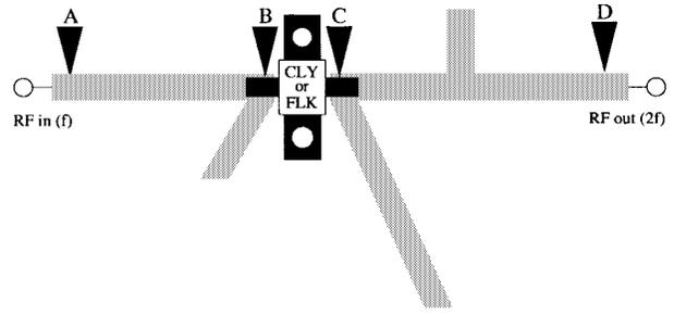
Fig. 8. General layout of frequency doublers showing locations of optical probing.
