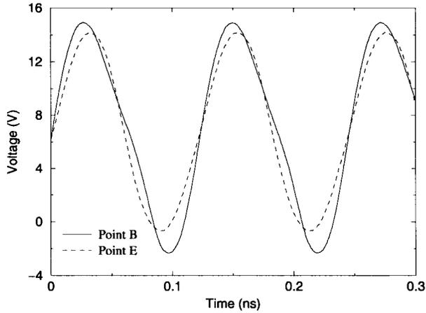
Fig. 6. Measured waveforms at points **B** and **E** in the class-E circuit. The shape of the voltage wave at **B** is similar to that in Fig. 6, with a second harmonic component in the waveform. The output wave at **E** is sinusoidal.
