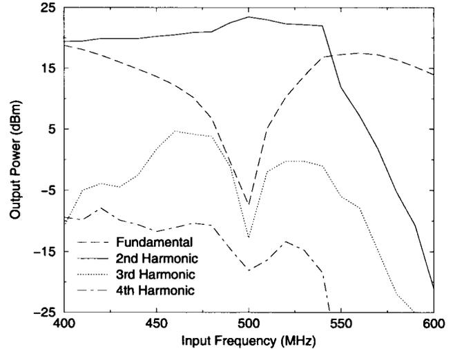
Fig. 9. Measured output power at the fundamental and first three harmonics versus input frequency for the 1-GHz doubler ( $P_{in} = 15$  dBm,  $V_{DS} = 5$  V, and  $I_{DS} = 110$  mA).
