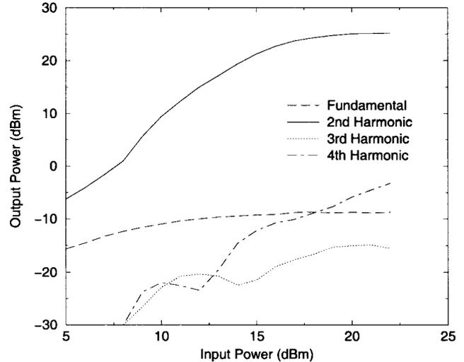
Fig. 12. Measured output power at the fundamental (2.5 GHz) and first three harmonics versus input power for the 5-GHz doubler ( $V_{DS} = 8$  V, and  $I_{DS} = 100$  mA).
