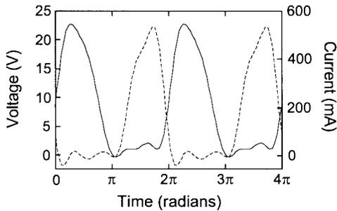
Fig. 7. Simulated waveform of a 500-MHz class-E circuit using a Materka-Kacprzak nonlinear model for a Siemens CLY5 MESFET. The solid line signifies voltage and the dashed line denotes current.
