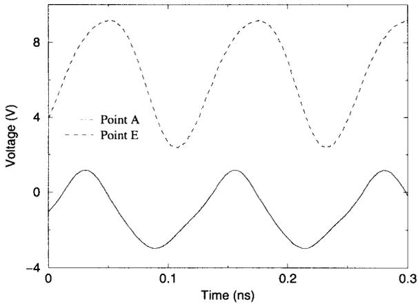
Fig. 4. Optically sampled waveforms at points **A** and **E** in the class-F circuit, corresponding to the input and output respectively. The input and output waveforms are both sinusoidal signals.
