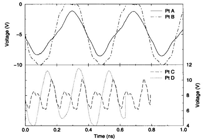
Fig. 13. Optically sampled waveforms at points A–D in the 2.56–5.12-GHz doubler.
