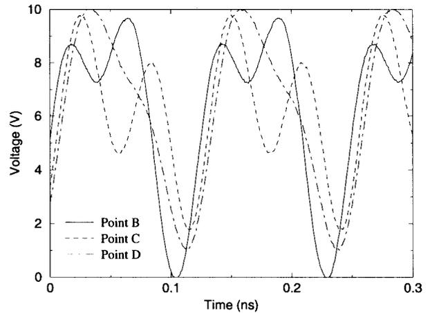
Fig. 5. Optically sampled waveforms at points **B**, **C**, and **D** in the class-F circuit. In the switch waveform at **B**, the fundamental and third harmonic approximate a square wave. At **C**, which is before the second harmonic shorting stub, there is a significant second harmonic component, and at **D**, the harmonics have mostly been filtered out. These waveform amplitudes cannot be used to calculate power since the local impedance is unknown.
