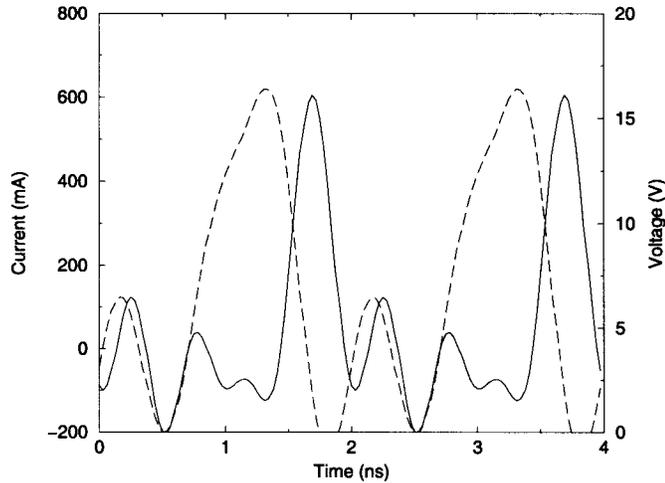
Fig. 10. Simulated drain voltage (solid line) and current (dashed line) waveforms for the 1-GHz doubler.
