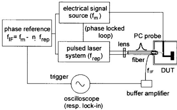
Fig. 2. Optical sampling measurement setup.
