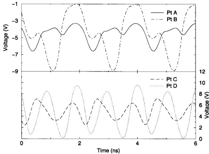
Fig. 11. Optically sampled waveforms at points A–D in the 480–960-MHz doubler.
