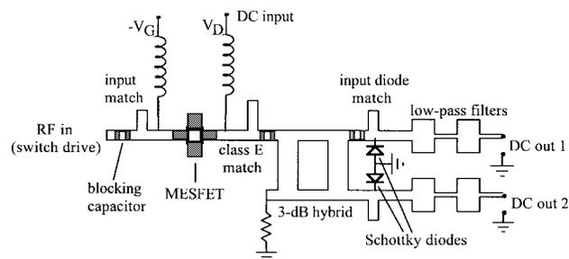
Fig. 1. Layout of the 4.5-GHz microwave dc–dc converter. The dc–ac part of the circuit is a class-E amplifier (or class-E oscillator), the output of which is divided between two half-wave diode rectifiers. The two dc outputs can be connected in series or parallel. The bias feeds are the part of the planar circuit.
