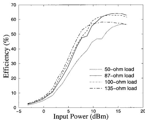
Fig. 5. Measured dc–dc conversion efficiency.
