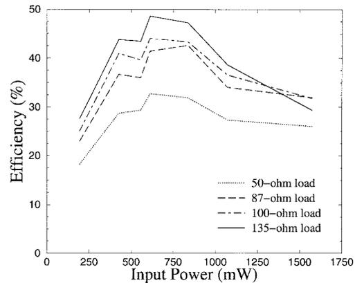
Fig. 7. Total dc–dc converter efficiency using class-E oscillator.
