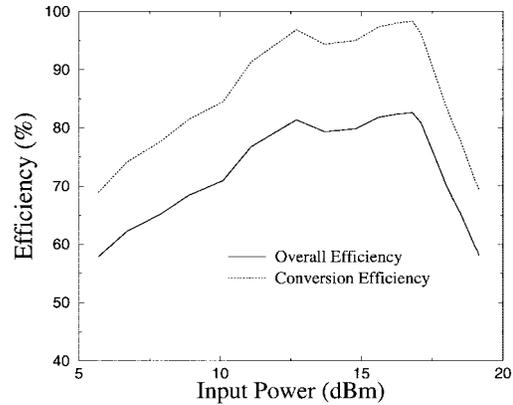
Fig. 3. Measured conversion and overall (total) efficiency of a single half-wave diode rectifier at 4.5 GHz, using a 135- $\Omega$  load. The lower curve includes the reflected wave due to input mismatch.
