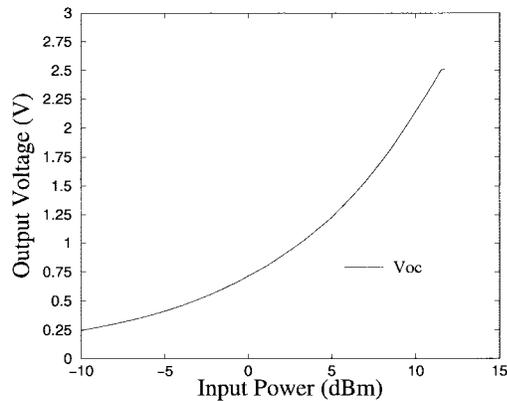
Fig. 4. Measured dc output open-circuit voltage as a function of input RF power.
