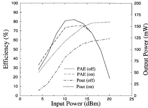
Fig. 2. Measured PAE and output power for a drain bias of 3 V. In one case, the transistor is biased for a drain current of 50 mA, and in the other, the gate is pinched off.
