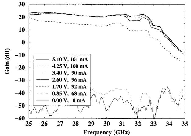
Fig. 7. Measured gain of the Alpha AA028P3-00 MMIC at various bias points.
