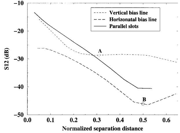
Fig. 3. Coupling is calculated as a function of normalized separation distance. The normalized separation distance is the shortest distance between the two elements divided by the slot antenna length. The circles correspond to the normalized distances used in the final array design.
