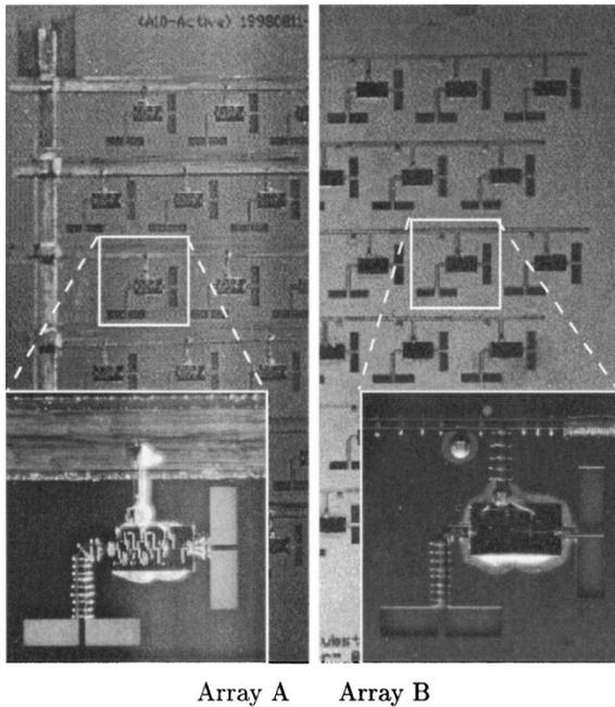
Fig. 6. Arrays *A* and *B* with corresponding unit cells enlarged. The size of the unit cell is 9 mm × 9 mm.
