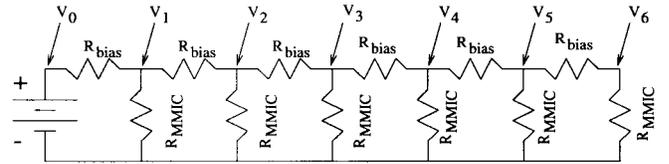
Fig. 4. Resistive ladder network diagram used to calculate MMIC bias levels within the array.
