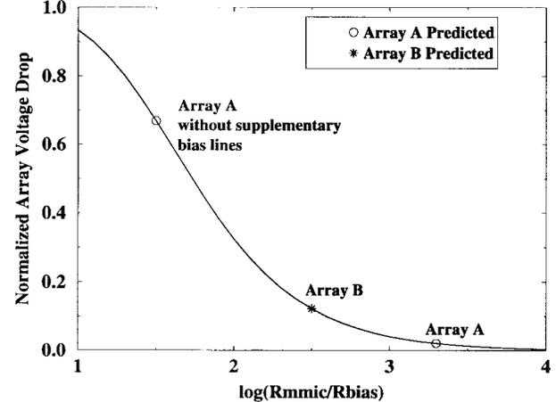
Fig. 5. Normalized array voltage drop as a function of  $R_{MMIC}/R_{bias}$ .
