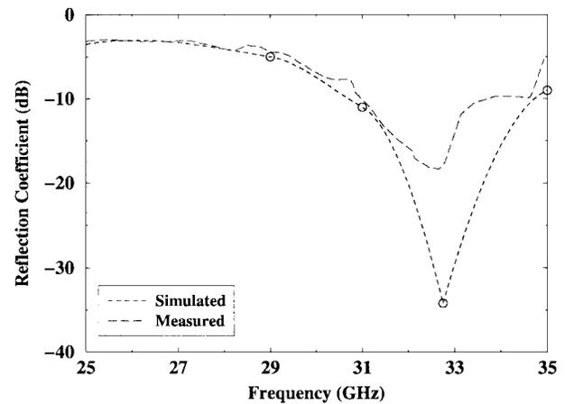
Fig. 8. Simulated and measured response of the slot antenna. HP Momentum was used for the simulation.
