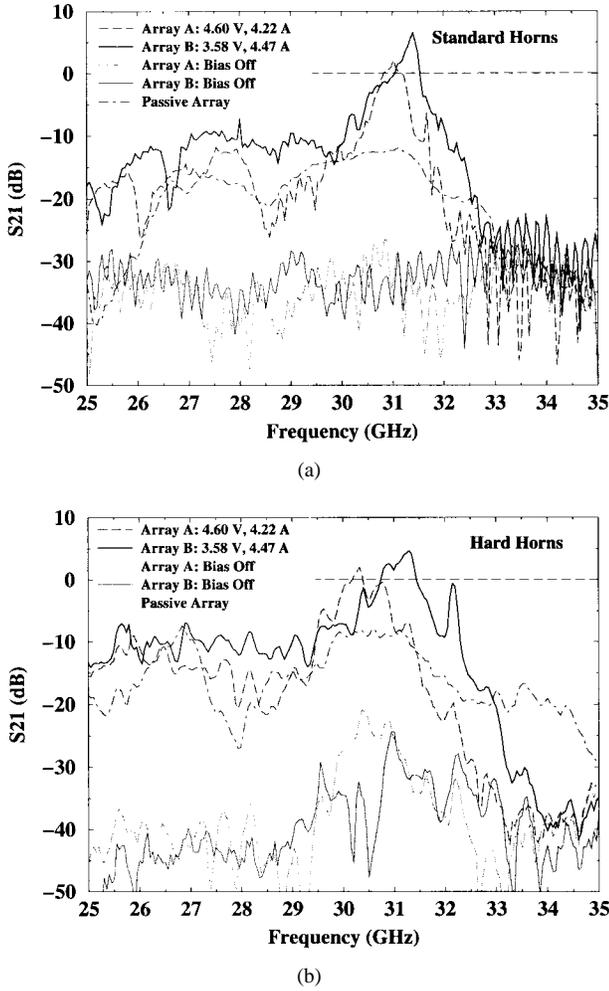
Fig. 9. Small-signal gain measurements with: (a) standard horns and (b) hard horns. Measurements are with respect to a through calibration.
