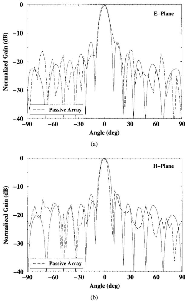
Fig. 10. (a) Passive *E*-plane pattern measurement. (b) Passive *H*-plane pattern measurement. The measurement frequency is 31.4 GHz. The theoretical plot (—) assumes a uniform array.
