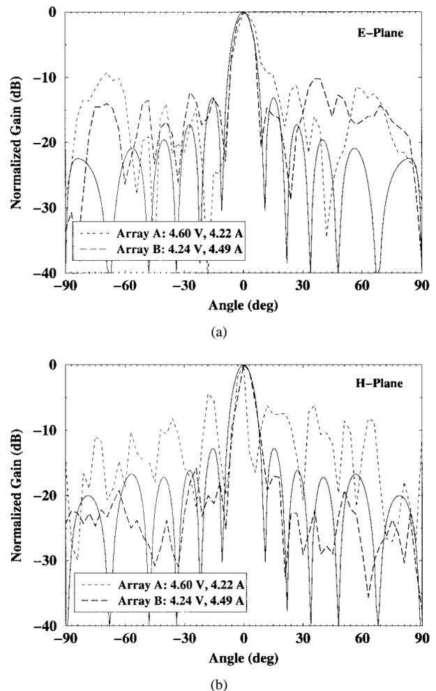
Fig. 11. (a) Active *E*-plane pattern measurement. (b) Active *H*-plane pattern measurement. The measurement frequency is 31.4 GHz. The theoretical plot (—) assumes a uniform array.
