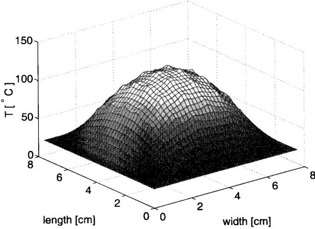
Fig. 2. Theoretical temperature on the surface of the AlN substrate is plotted as a function of position. The spikes in the temperature distribution are due to the finite area of individual MMIC's.
