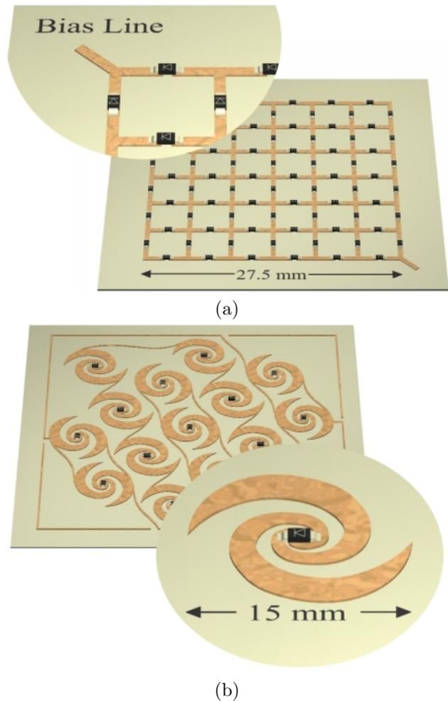
Fig. 1. The grid (a) and spiral (b) arrays. The latter is arrayed as alternating RHCP and LHCP elements, while the former rectifies one half cycle of both polarizations equally.
