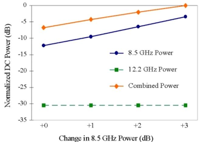
Fig. 4. Measured normalized DC power for a vertically polarized incident wave at 8.5 GHz (circular symbols), at 12.2 GHz (square symbols), and for waves at both frequencies simultaneously (diamond symbols). In the latter case the DC measured power is increased by 3 to 5 dB over the simple sum of the first two cases.
