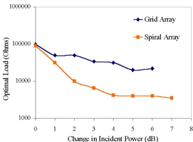
Fig. 5. Measured optimal load for maximum DC power transfer as a function of incident power for both the grid and the spiral rectenna arrays.
