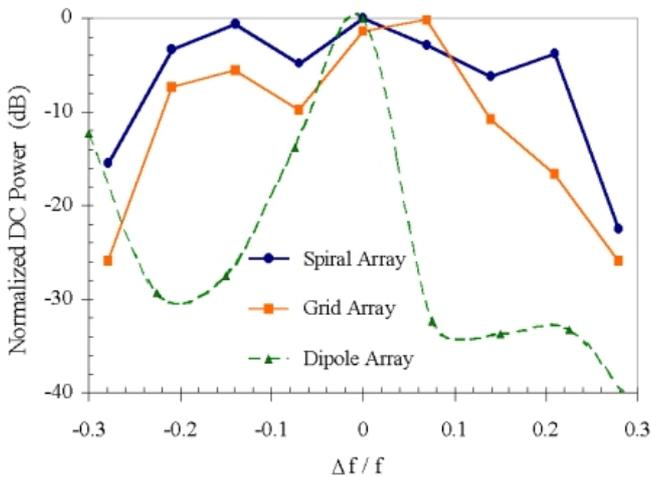
Fig. 3. Measured frequency response of normalized DC power delivered to an optimal load for the grid rectenna array (square symbols), spiral array (circular symbols) and linear 8-element resonant dipole array (triangular symbols). The response is measured with an incident circularly polarized wave at boresight.
