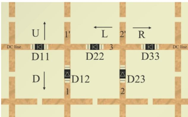
Fig. 2. Schematic of a portion of the grid rectenna array used in the explanation of the physical principles of operation.
