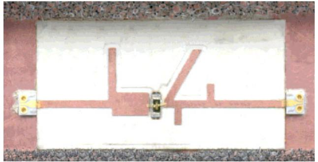
Fig. 1. Photograph of the fabricated 10.4/20.8 GHz multiplier circuit. The  $50\ \Omega$  transmission lines are 0.4 mm wide.
