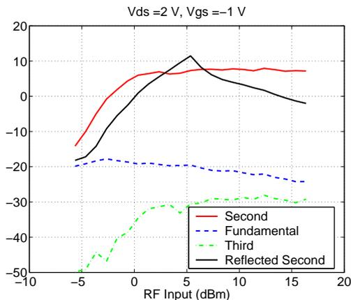
Fig. 4. Measured output and reflected power of the 20.8 GHz doubler as a function of input RF power.
