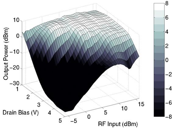
Fig. 3. Measured output power of the 20.8 GHz doubler vs. drain bias and RF input power for  $V_{gs}=1$  V. There is no significant increase in output power as the drain voltage is increased.
