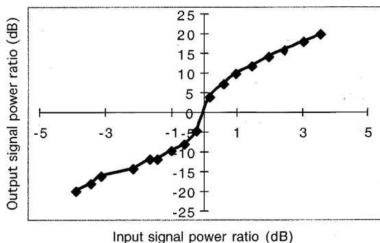
Fig. 11. Measured signal enhancement provided by the auto-tuning filter. We define signal enhancement as the power ratio of the two signals at the output divided by their power ratio at the input.
