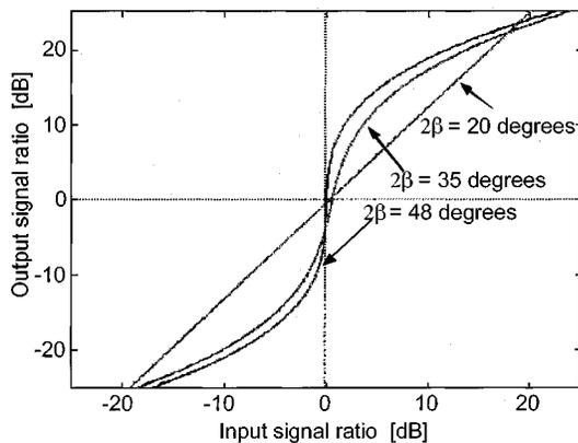
Fig. 15. Signal extraction properties of the adaptive system parameterized by the mutual angle between the transmitters.
