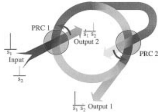
Fig. 10. Schematic diagram of the auto-tuning filter. Two photorefractive crystals (PRCs) are interconnected in a reflexive oscillator configuration. The strongest independent component of the ensemble of input signals is extracted at Output 1 while the remainder appear at Output 2.
