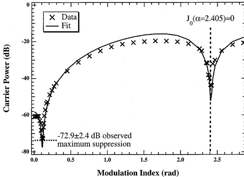
Fig. 9. Measured performance of carrier suppression by two-beam coupling (crosses) and comparison with theory (solid curve).
