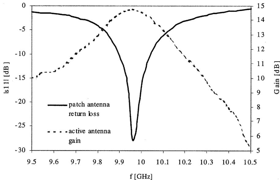
Fig. 5. Measured return loss of receiver patch antenna (solid line) and gain of active antenna at the output of the LNA (dashed line).
