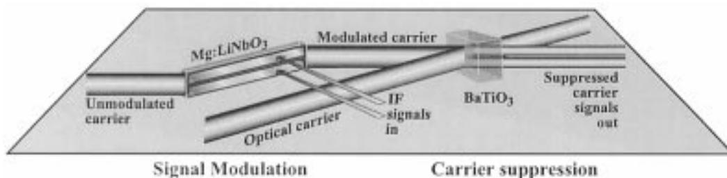
Fig. 6. Schematic of the EOM and carrier suppression circuits.
