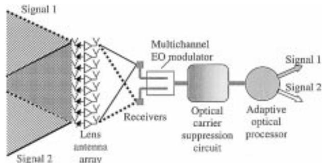
Fig. 1. Block diagram of the optically smart antenna array with two sources in the far field. The active receivers are positioned on the focal arc of the discrete lens antenna. The IF signals are then imposed onto the optical beam and processed by the adaptive optical circuit.
