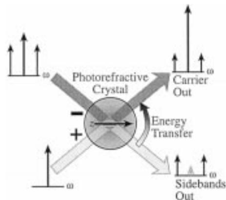
Fig. 7. Schematic diagram of two-beam coupling carrier suppression. The input to the minus (“-”) port is a modulated laser beam while the input to the plus (“+”) port is an unmodulated beam from the same laser. Nonlinear coupling between the beams causes the energy in the carrier at the minus port to be transferred to the plus port at the output.
