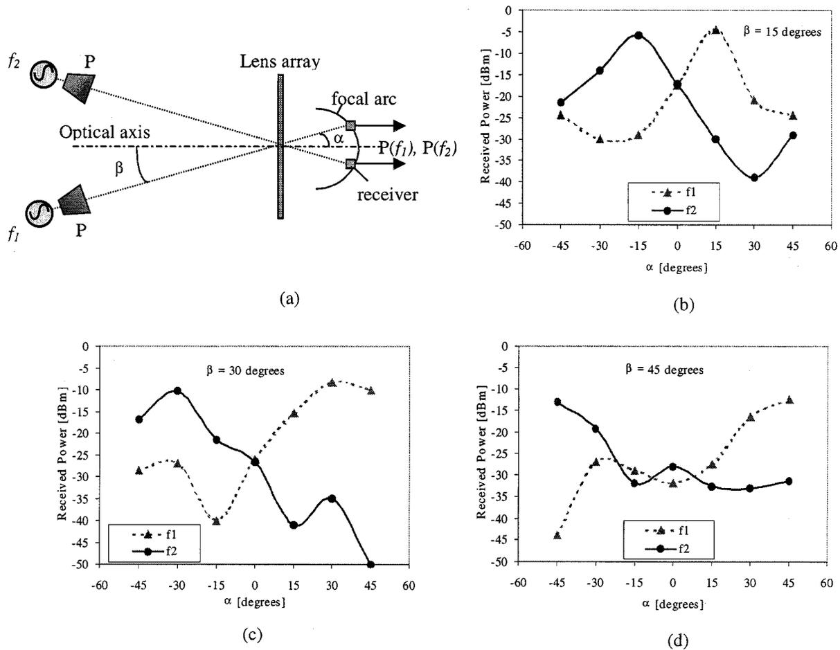
Fig. 3. (a) Schematic of measurement setup used to characterize the multiple-receiver lens antenna array. Each transmitting antenna is located 0.8 m from the lens and transmits 25 dBm at frequencies 10 MHz apart around 9.9 GHz. Measured “crosstalk” between the two signals as a function of the receiver position along the focal arc ( $\alpha$ ) for different transmitter position. (b)  $\beta = 15^\circ$ . (c)  $\beta = 30^\circ$ . (d)  $\beta = 45^\circ$ .
