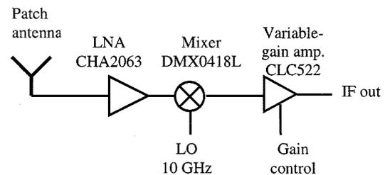
Fig. 4. Block diagram of receiver positioned on the focal surface of the lens array.
