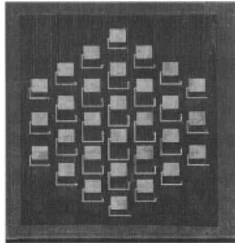
Fig. 2. Photograph of one side of a 30-element X band two-layer quasi-optical lens antenna array with patch antenna elements. The array lattice is triangular with an element size of 0.63 by 0.83 free-space wavelengths at 10 GHz. The feed lines vary in length across the array, producing a focal surface. The feed lines are connected with via holes to orthogonally polarized patch antennas on the other side of the two-layer array.
