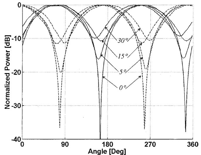
Fig. 12. Measured polarization properties for the two polarization states of the lens for four scan angles ( $0^\circ$ ,  $5^\circ$ ,  $15^\circ$ , and  $30^\circ$ ) as the transmitting horn polarization is rotated.
