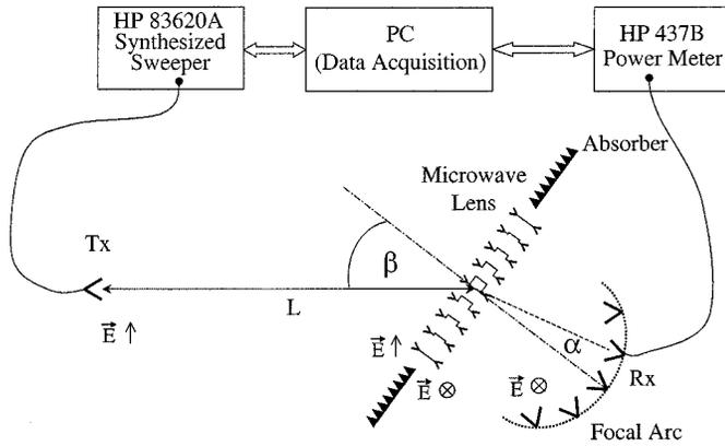
Fig. 7. Sketch of measurement setup used to characterize the lens array. A standard-gain linearly polarized far-field horn antenna is used as a transmitter and another horn antenna is used at the receive port.
