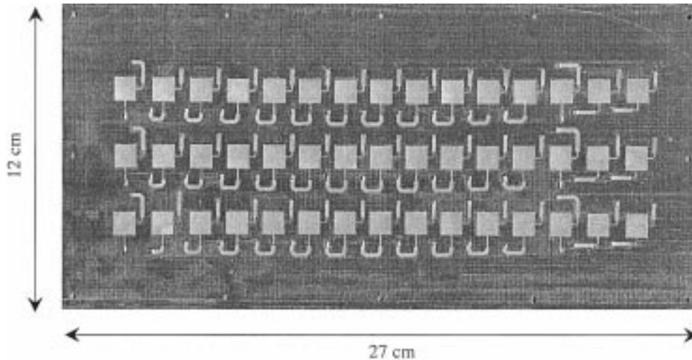
Fig. 2. Photograph of one side of a 45-element 10-GHz cylindrical lens antenna array shows the patch antenna elements with dual-polarization feed lines and the microstrip delay lines connected with via holes to orthogonally polarized patches on the other side of the two-layer lens array.
