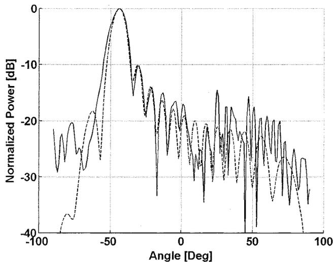
Fig. 11. Calculated (dashed) and measured (solid) lens array radiation patterns for a beam steered to  $-45^\circ$ .
