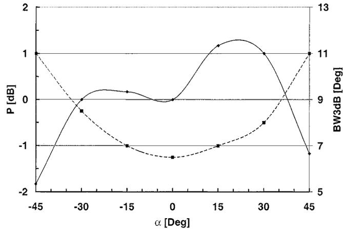
Fig. 9. Measured received power (solid line) and half-power beamwidth (dashed line) as the receiver is moved along the lens focal arc, normalized to the power level received on the optical axis.
