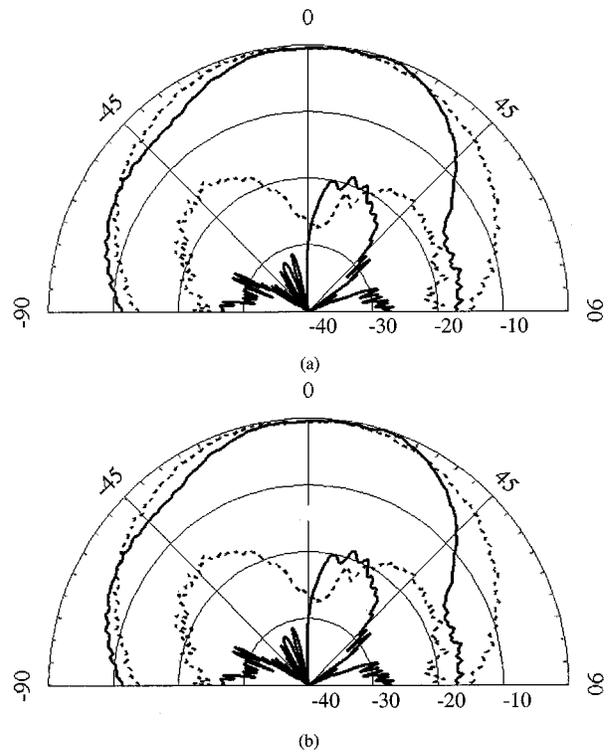
Fig. 5. Measured element E-plane (solid) and H-plane (dashed) co- and cross-polarized radiation patterns for the two orthogonally polarized ports, (a) and (b).
