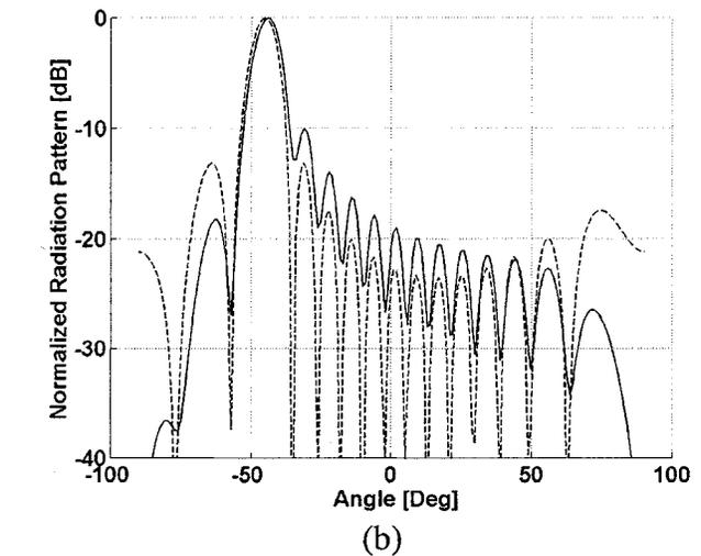
Fig. 10. Calculated lens array radiation patterns with the corresponding amplitude distributions and path-length errors, for a beam at boresite (a), and steered to  $-45^\circ$  (b). Dashed lines represent the case for uniform amplitude distribution and the receiving antenna at a distance  $F$  from the lens array. Solid lines represent the case with the actual amplitude distribution and the receiving antenna at the optimal focal arc.
