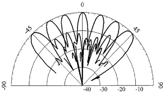
Fig. 8. Measured normalized multibeam patterns for receivers (or transmitters) positioned at points along the focal arc corresponding to beams at  $-45^\circ$ ,  $-30^\circ$ ,  $-15^\circ$ ,  $0^\circ$ ,  $15^\circ$ ,  $30^\circ$ , and  $45^\circ$ . Sidelobe levels for a beam steered to  $-45^\circ$  are shown in more detail as compared to simulations in Fig. 11.
