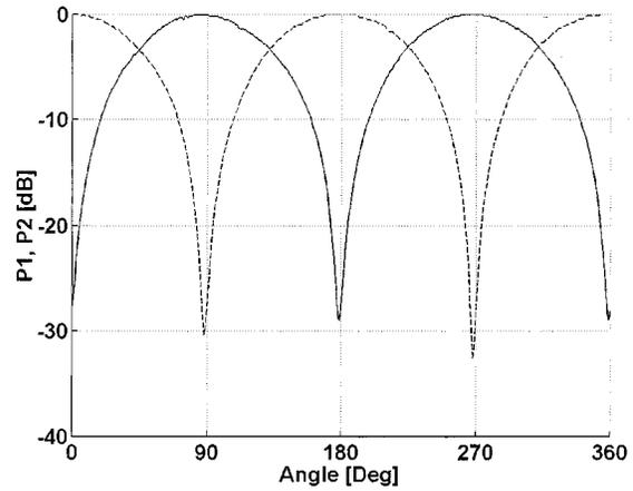
Fig. 6. Measured axial ratio of array element for the two orthogonally polarized feeds. The solid and dashed lines are the measured relative powers received at the two ports of the element as the transmitting horn polarization is rotated.
