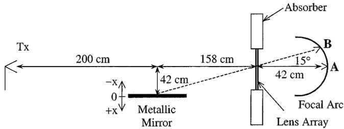
Fig. 13. Multipath measurement setup with a single  $15 \times 15$  wavelength reflector which is translated by three wavelengths in the  $x$  direction. The  $x = 0$  reference level corresponds to the second null in the lens radiation pattern, as shown in Fig. 10(a).
