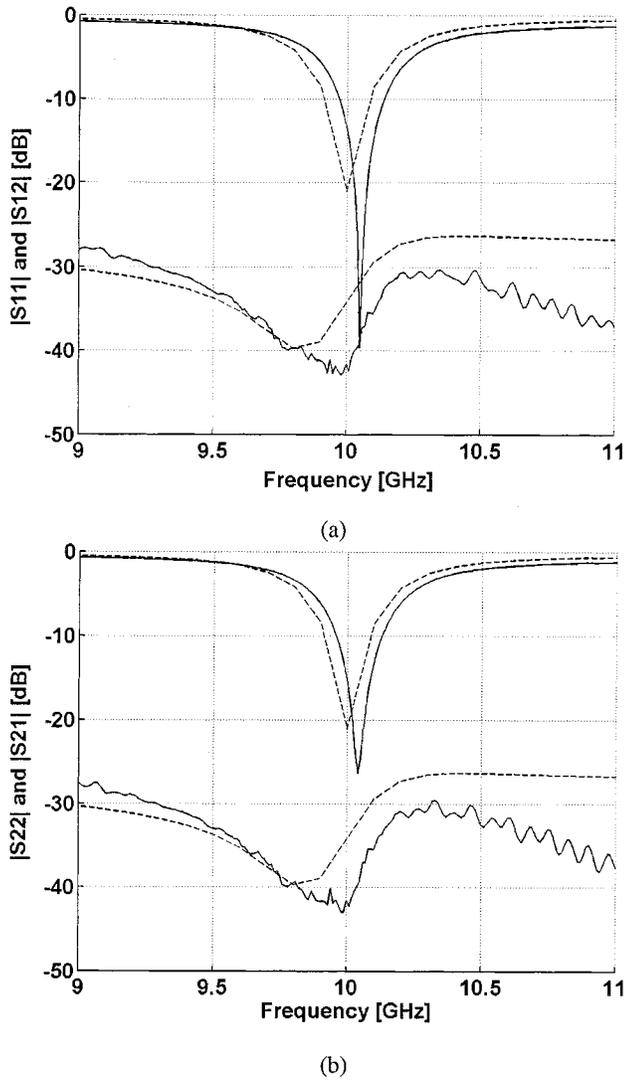
Fig. 4. Measured (solid line) and simulated (dashed line) two-port unit cell *s*-parameters, where the ports correspond to orthogonally polarized feeds.
