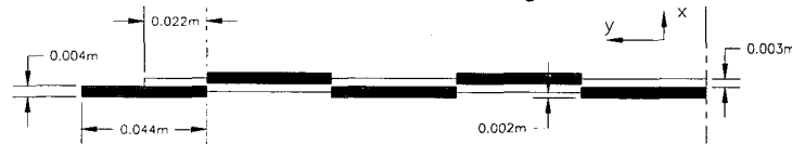
Figure 1: Left half of 10-element planar OPOMEX antenna geometry [1]. Antenna is skew symmetric about the vertical centerline.
