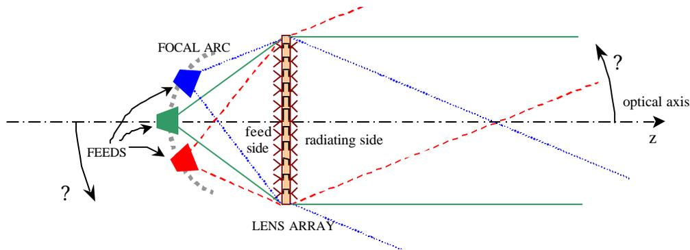
Fig. 1. Schematic of a planar discrete lens array with several independent feeds on its focal arc. Each feed controls a radiation pattern with the main beam pointing at a different angle off boresite.
