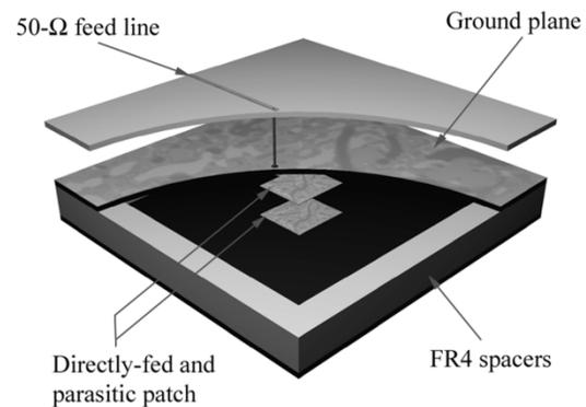
Fig. 5. Schematic of the broad-band patch antenna. Patches are machined on a low-cost Rogers Ultralam 2000 substrate, with  $\epsilon_r = 2.43$ , 0.483-mm thick. The vertical distance between patches is 2.93 mm. The feed shares the common ground plane with the directly fed patch. It is shown separated from the patch layer for clarity.
