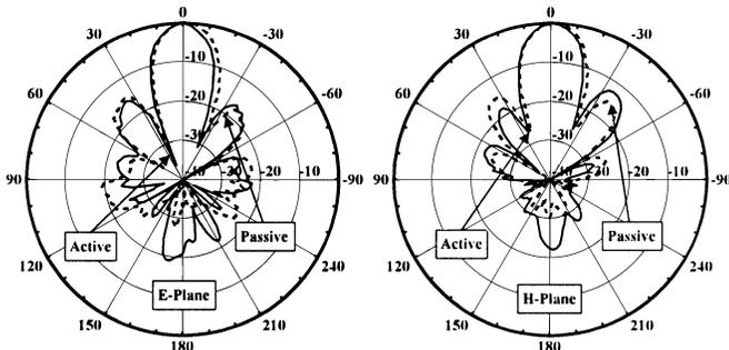
Fig. 13. Radiation patterns of the passive (dashed line) and active (solid line) 16-element antenna array at 10.2 GHz.
