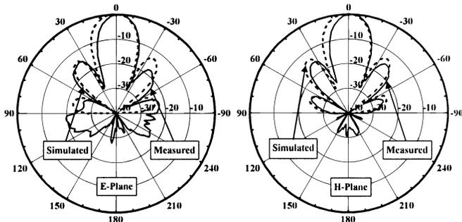
Fig. 12. Simulated and measured radiation patterns of the passive 16-element antenna array at 10.2 GHz.
