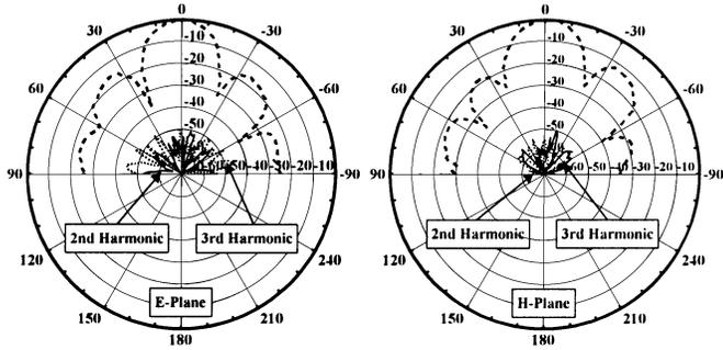
Fig. 16. Second harmonic (solid line) and third harmonic (dotted line) radiation patterns of the active 16-element array operating at 10.2 GHz.
