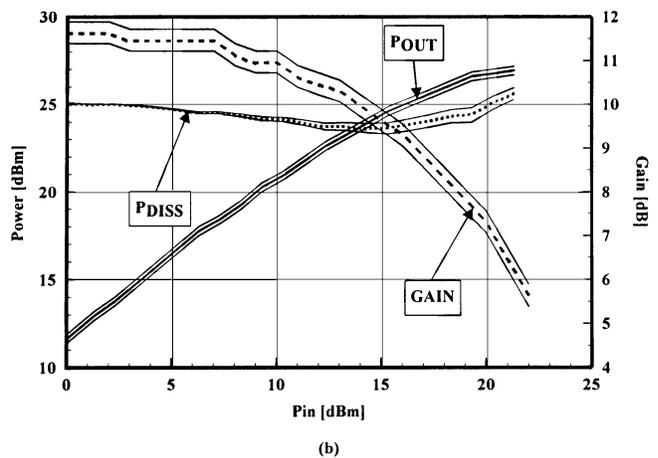
Fig. 10. Power sweep characteristics of the amplifier stage in the four-element active subarray. The bounds on performance correspond to an estimated 0.5-dB uncertainty in output power measurement. The PAE shown in (b) does not include the feed loss.
