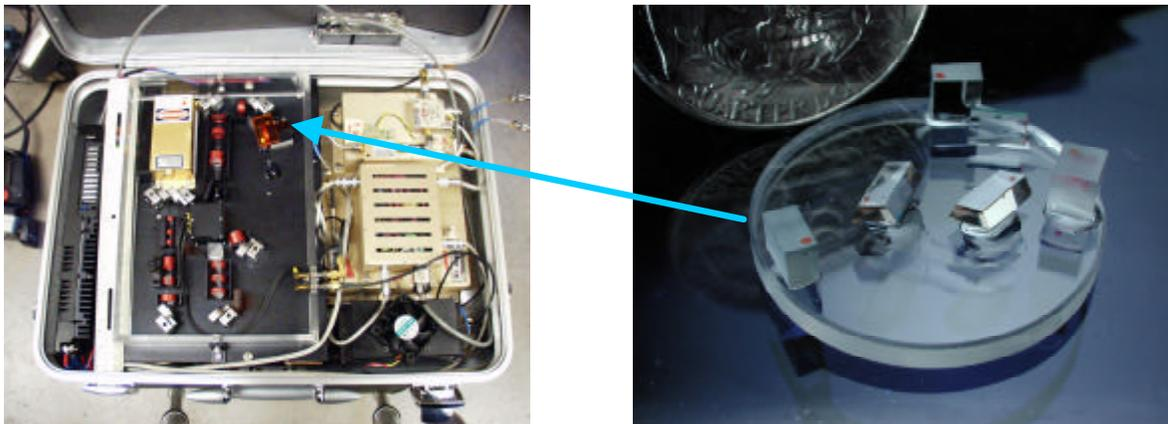
**Figure 4.** Photographs of integrated PCA smart antenna array processor in standard-size briefcase (left) and the optical processor integrated on a glass coin the size of a US quarter (right).
