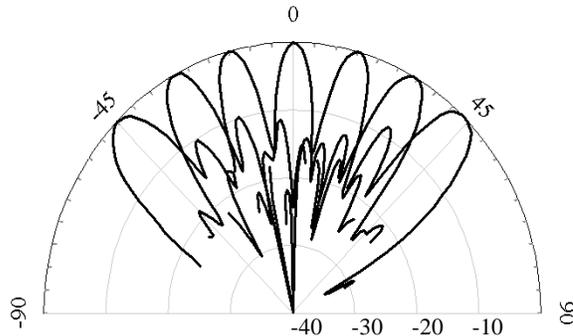
**Figure 2.** Measured multibeam patterns of a 10-GHz DLA optimized for wide scan angles. The peak power varied by  $\pm 1$ dB, and the beamwidth by a few degrees over the 90-degree scan range.
