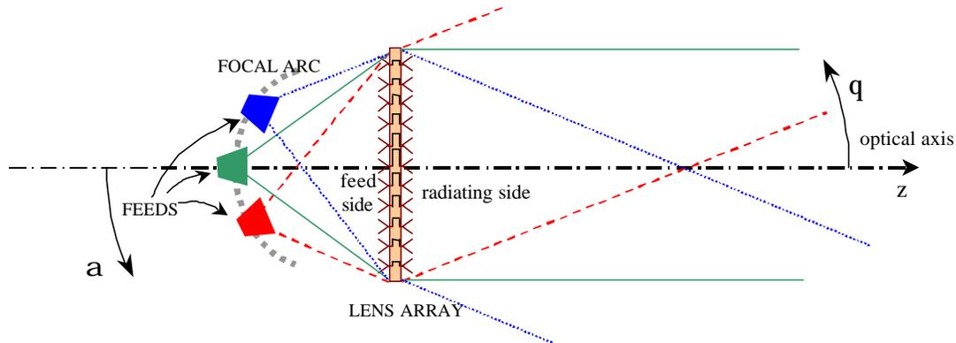
**Figure 1.** Sketch of a discrete lens array.
