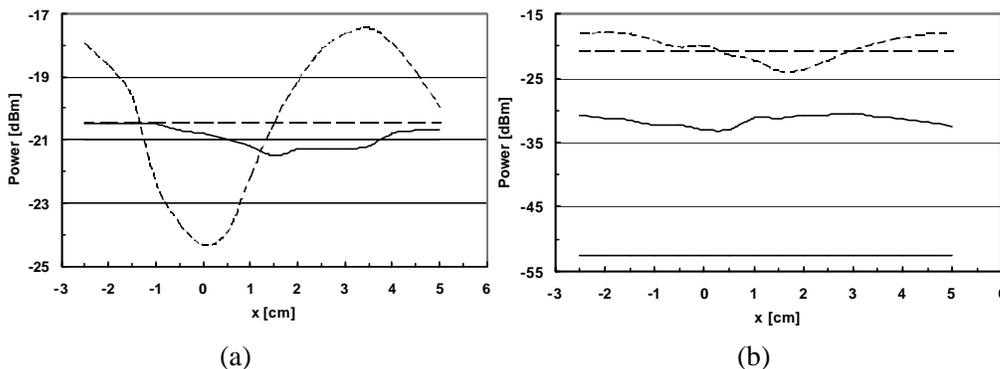
**Figure 3.** Measured received co-polarized power in the presence of controlled multipath without lens in link (dashed line) and with the lens added at the front end of the receiver (solid line). The receiver is positioned for a beam at 0 degrees (a) and 15 degrees (b). The straight lines show the reference power levels received with no reflector (no multipath) in the link, for 500mW input power to the transmitting horn antenna in a line-of-sight setup.
