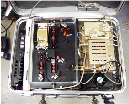
Fig.1. Photograph of integrated PCA smart antenna array processor. The antenna feeds are the cables on the righthand side. A single 110-V plug supplies the required 50W of power to all the optical and electronic parts of the system. The package is a standard size briefcase.
