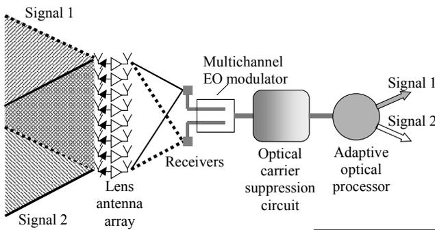
Fig.2. Block diagram of the PCA system from Fig.1, consisting of the microwave antenna and receivers, followed by the EO modulator, optical carrier suppression and optical processor.
