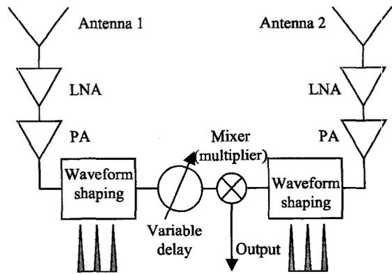
Fig. 2. Block diagram of angle-of-arrival detection system with nonlinear signal processing. In this paper, the system was implemented at 2GHz with low-cost off-the-shelf components.
