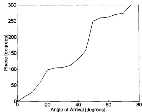
Fig.5. Measured phase shift in the feed of one element of a to-element at 2GHz required to determine directions of arrival for plane waves from 0 to  $90^\circ$  with a receive E-plane directivity corresponding to a 5-element array.
