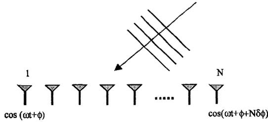
Fig. 1.  $N$ -element antenna array with incident plane wave.
