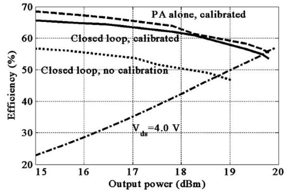
Fig. 9. Measured efficiency for the PA with constant drain bias (dashed–dotted line), the PA with manual drain bias control (dashed line), the entire closed-loop system when the connector loss and coupler loss is calibrated out (solid line), and the uncalibrated closed-loop system (dotted line).
