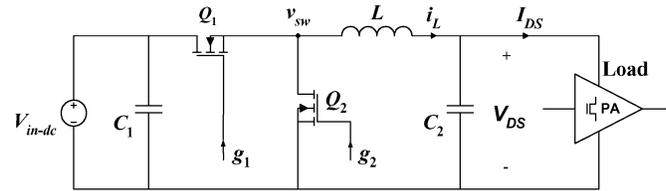
Fig. 5. Power stage of the synchronous buck converter. The range of input dc voltage is 5–7 V,  $C_1 = C_2 = 10 \mu\text{F}$ ,  $L = 10 \mu\text{H}$ , and the load is the class-E microwave PA drain terminal. The MOSFETs used in this implementation are IRF7331.
