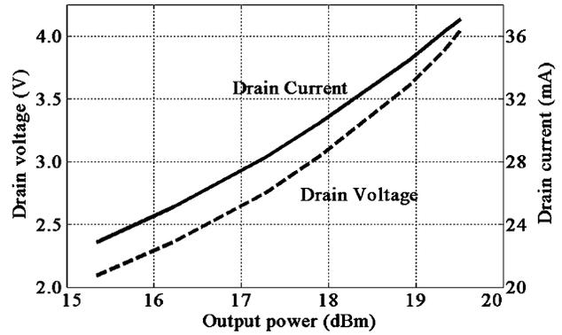
Fig. 4. Measured drain voltage and current of the PA versus output power for constant input power.
