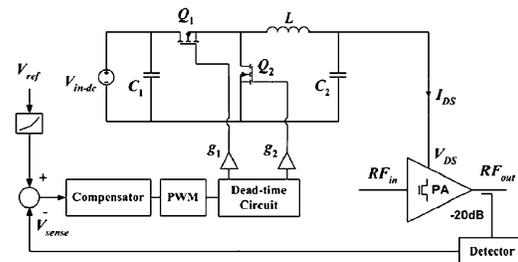
Fig. 1. Switched-mode PA with closed-loop power control using dynamic drain bias.
