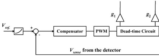
Fig. 6. Self-assessment signal  $V_{\text{sense}}$  from the detector at the output of the PA is compared with a pre-measured power reference signal  $V_{\text{ref}}$  obtained by characterizing the PA. The PWM generates the gate-drive control signals  $g_1$  and  $g_2$  for the MOSFETs  $Q_1$  and  $Q_2$  from Fig. 1.
