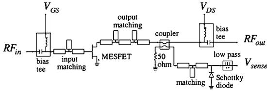
Fig. 2. Microwave portion of the dynamically controlled PA circuit, includes the PA with input and output matching circuits, biasing circuits, and output power detector (coupler, Schottky diode, and low-pass filter).
