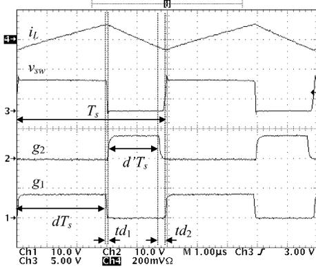
Fig. 7. Measured waveforms in the synchronous buck converter. Trace 1: gate drive signal  $g_1$ . Trace 2: gate drive signal  $g_2$ . Trace 3:  $Q_2$  drain voltage  $v_{\text{sw}}$ . Trace 4: inductor  $L$  current  $i_L$  (200 mA/div). The switching frequency is  $f_s = 200$  kHz with an output voltage  $V_{\text{DS}} = 3$  V and load current  $I_{\text{DS}} = 30$  mA.
