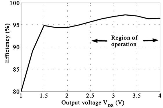
Fig. 8. Measured efficiency of the dc–dc converter as a function of the output voltage  $V_{\text{DS}}$  for the PA as the load.
