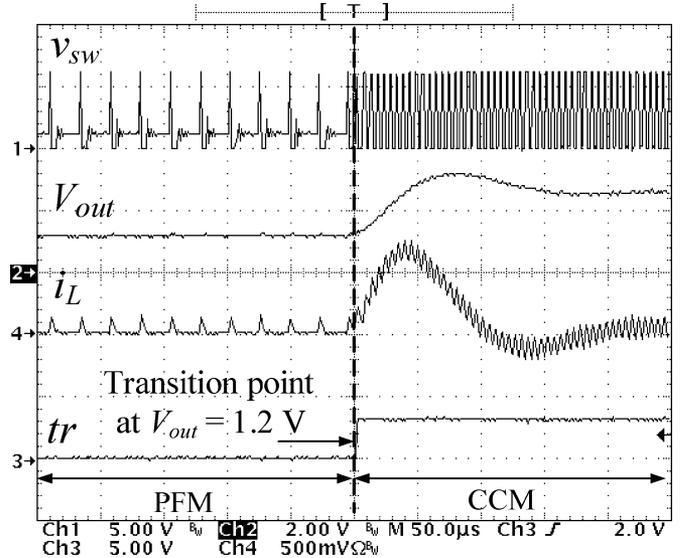
Fig. 15. Switching voltage  $v_{sw}$ , the output voltage  $V_{out}$ , the inductor current  $i_L$ , and the mode logic signal (high = CCM, low = PFM) in the experimental digitally controlled buck converter. The mode switching occurs at  $V_{out} = 1.2$  V.
