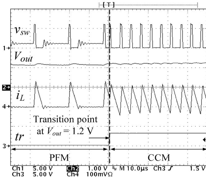
Fig. 14. Switching voltage  $v_{sw}$ , the output voltage  $V_{out}$ , the inductor current  $i_L$ , and the mode logic signal (high = CCM, low = PFM) in the experimental digitally controlled buck converter. The mode switching occurs at  $V_{out} = 1.2$  V. The initial value of the duty ratio in the first CCM cycle after the transition from PFM is programmed to minimize the disturbance in the output voltage.
