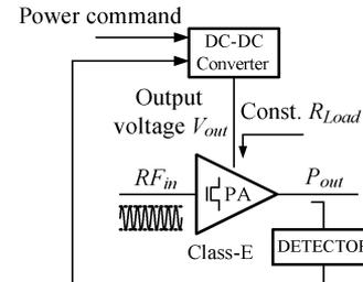
Fig. 1. System block diagram: RF power amplifier (RFPA) is supplied from a dc/dc converter. The converter and the RFPA form a closed-loop power control system where the supply voltage  $V_{out}$  to the RFPA is adjusted so that the sensed RF output power matches the power command.
