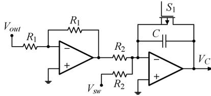
Fig. 11. Details of the current estimator circuit.
