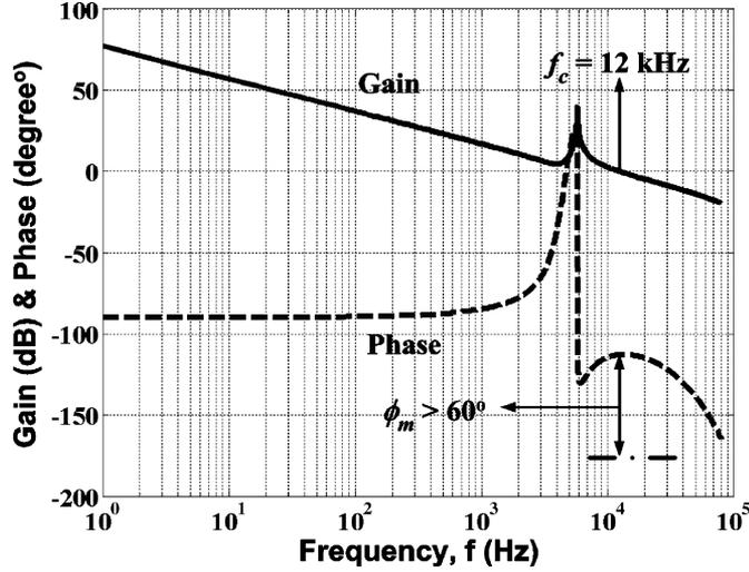
Fig. 10. Magnitude and phase responses of the loop gain for the digitally controlled buck converter operating in CCM.
