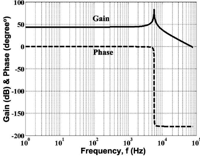
Fig. 9. Bode plots of the control to output transfer function of the buck converter operating in CCM.  $L = 30 \mu\text{H}$ ,  $C = 25 \mu\text{F}$ .
