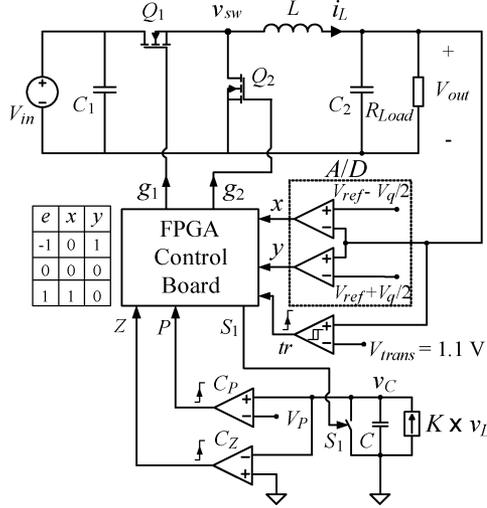
Fig. 7. Experimental test circuit.
