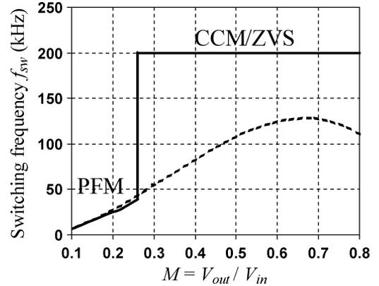
Fig. 5. Measured converter switching frequency (solid line) and the PFM switching frequency found from (3) (dashed line) as functions of the conversion ratio  $M = V_{out}/V_{in}$ .
