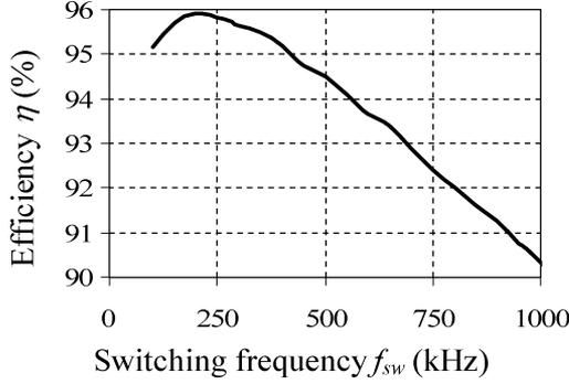
Fig. 2. Experimental efficiency of the dc/dc converter as a function of the switching frequency  $f_{sw}$ .
