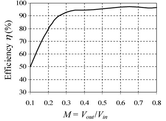
Fig. 3. Experimental efficiency of the dc/dc converter operating in CCM, as a function of the conversion ratio,  $M = V_{out}/V_{in}$ .
