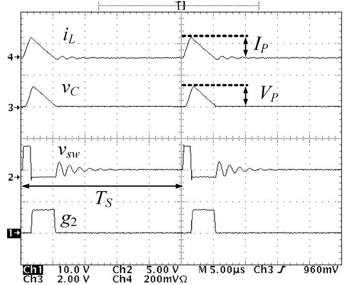
Fig. 12. Measured waveforms in the synchronous buck converter operating in PFM.  $I_P = 120$  mA,  $V_P = 1.2$  V,  $V_{in} = 5$  V,  $V_{out} = 1$  V,  $f_{sw} = 40$  kHz.
