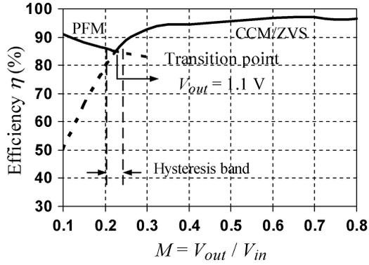
Fig. 4. Measured converter efficiency as a function of the conversion ratio  $M = V_{out}/V_{in}$ , for two modes of operation: PFM and CCM.
