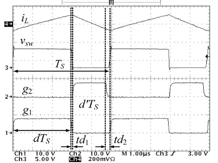
Fig. 8. Measured waveforms in the synchronous buck converter operating in CCM.  $V_{in} = 5$  V,  $V_{out} = 3$  V,  $f_{sw} = 200$  kHz.
