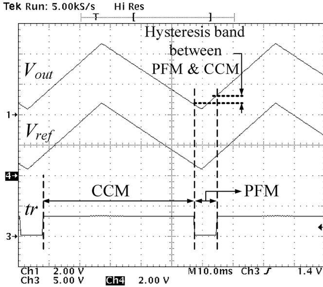
Fig. 13. The output voltage  $V_{out}$ , the reference voltage  $V_{ref}$ , and the mode logic signal (high = CCM, low = PFM) in the experimental digitally controlled synchronous buck converter.
