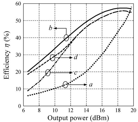
Fig. 16. Experimental system efficiency results: (a) RFA is supplied from a constant voltage  $V_{DS}$ , (b) the supply voltage of the RFA,  $V_{DS}$  is varied dynamically from an ideal 100% efficient power supply, (c) the RFA is supplied by the dc/dc converter operating in CCM over the entire range of output power, and (d) the RFA is supplied by the dual-mode PFM/CCM dc/dc converter.
