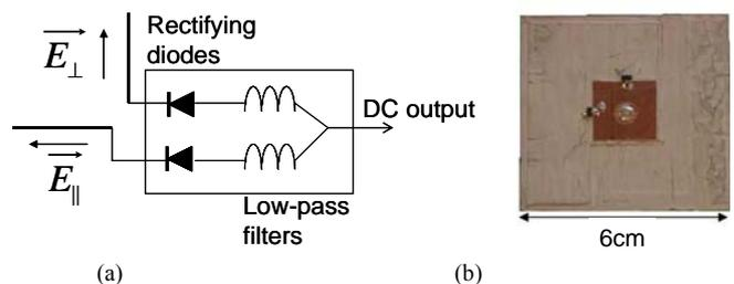
Fig. 2 (a) Block diagram of a dual-polarized rectenna and (b) photograph of a 2.4GHz dual-polarized patch rectenna. Two rectifying diodes are connected to the orthogonally polarized radiating edges of the patch, and the DC power is extracted through the via positioned at the RF voltage null of the antenna.
