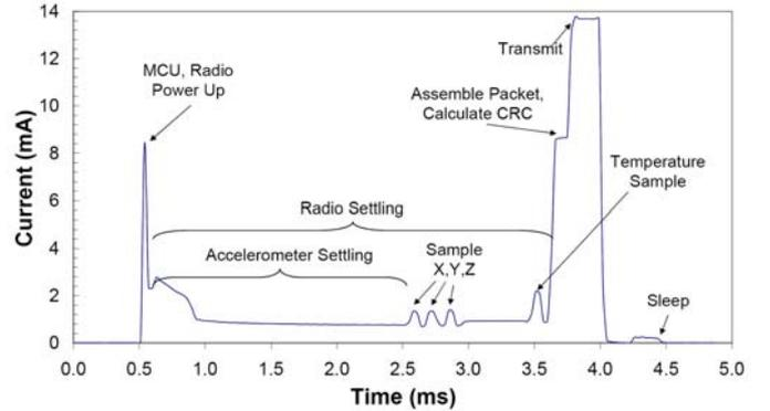
Fig. 6. Sensor module power consumption during one sample-and-transmit cycle. The graph shows the wake-up and settling period of the microcontroller (MCU) and various onboard sensors. The MCU samples and wirelessly transmits sensor data within 4 ms, after which it returns to a low-power ‘Sleep’ state.
