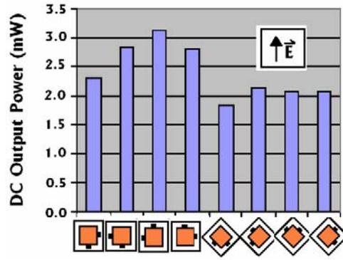
Fig. 4 Measured histogram of DC power levels for an incident power level of  $170 \mu\text{W}/\text{cm}^2$  for different orientations of the dual-polarized rectenna element, corresponding to different incident polarizations. The incident RF power is linearly polarized.
