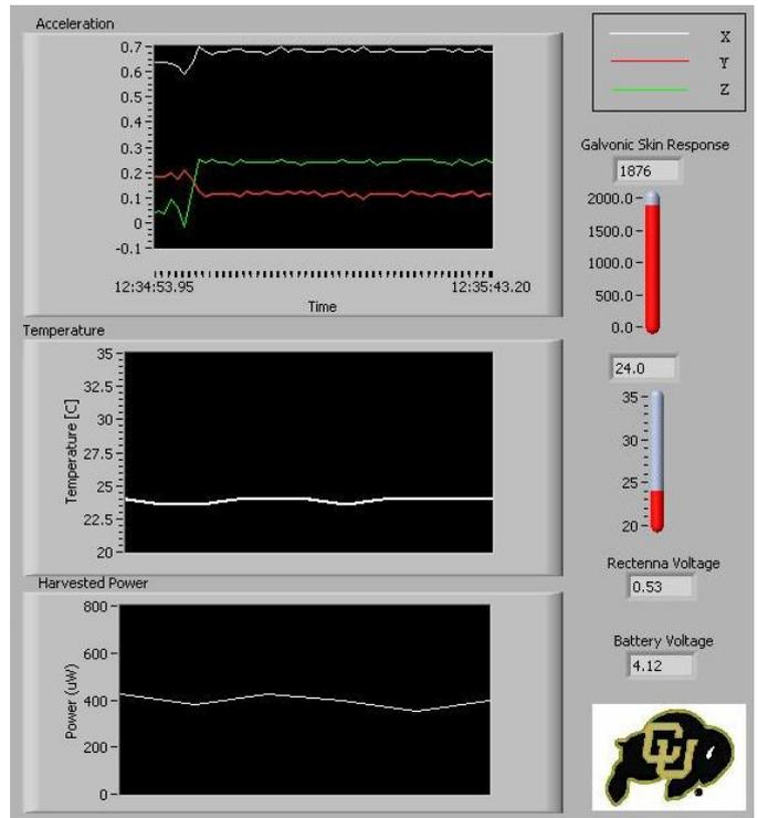
Fig. 9 User interface designed in LabVIEW that reports all data being collected and transmitted by the wirelessly-powered wireless sensor platform.
