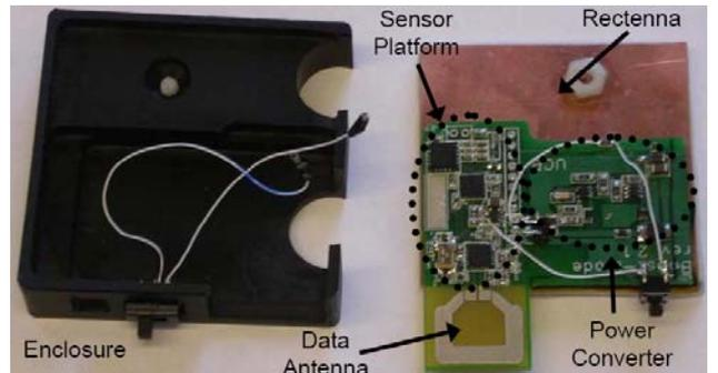
Fig. 7 Photograph of wirelessly powered wireless sensor. The power converter, sensors, controller and transceiver are integrated onto a single PCB and mounted directly above the rectenna with connections underneath the PCB. The separate data-transmitting antenna is a short folded dipole. The size of the package is 6cm x 6cm x 0.8cm.
