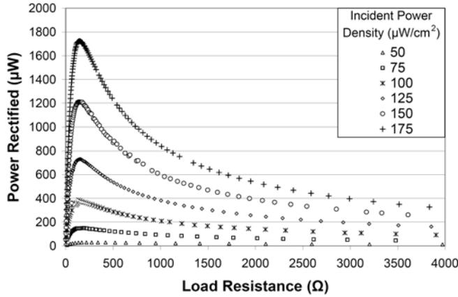
Fig. 3 Measured output DC power from a rectenna as a function of DC load resistance over a range of low-level incident power densities. The incident plane wave is linearly polarized along one of the two patch edges.
