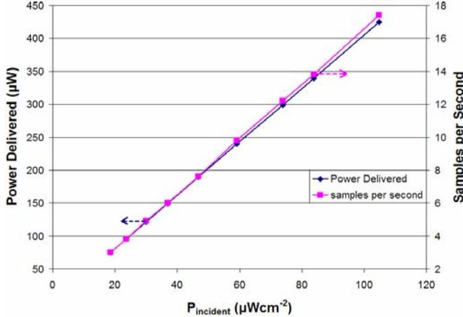
Fig. 8 Power delivered from the converter and the corresponding maximum samples per second for given incident RF power level such that there is no net power consumption.
