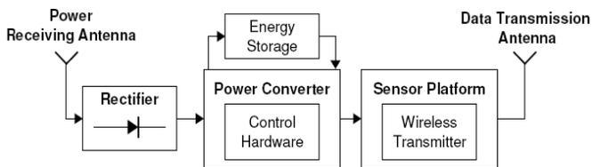
Fig. 1 Block diagram of wirelessly-powered low-power wireless sensor. Sensors collect data which is then transmitted from a low-power wireless transmitter. Power is received through RF waves incident on a powering antenna integrated with a rectifier (rectenna). A digitally-controlled power-management circuit optimally charges an energy storage device which provides power to the sensor platform.
