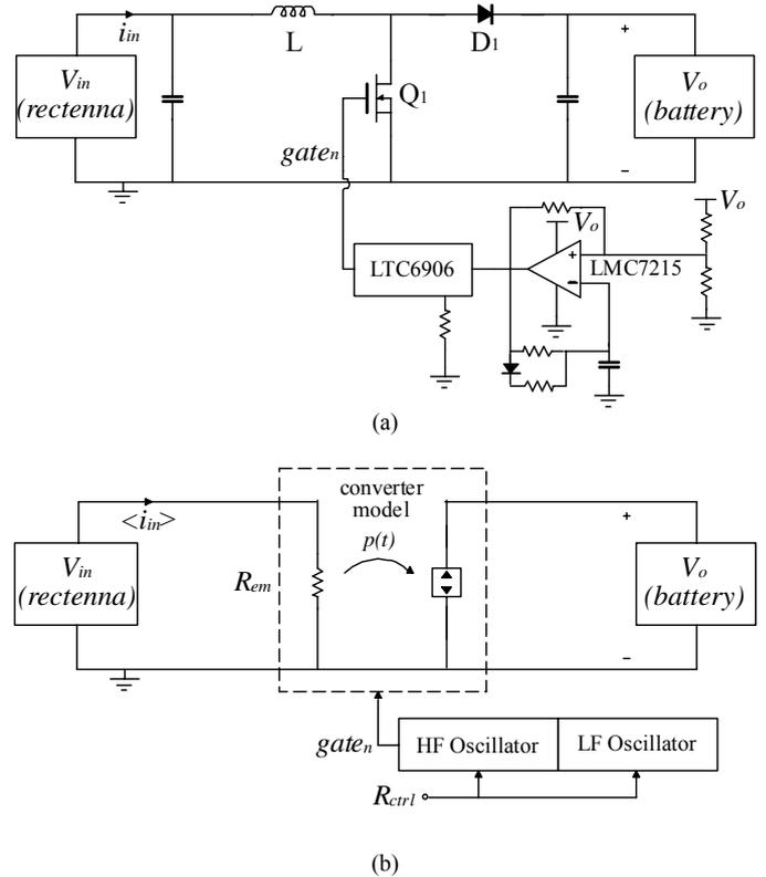
Fig. 5. (a) Boost converter schematic with simplified control circuitry to achieve near constant resistor emulation. (b) Block diagram of converter model and associated control.
