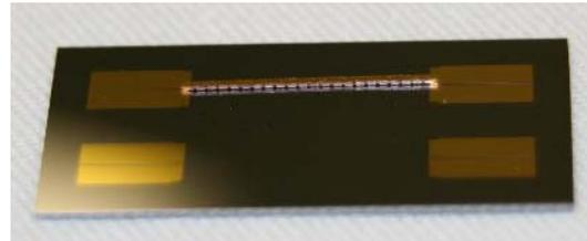
Fig. 6. Photograph of a 1-cm micro-rectangular coaxial transmission line flip-chipped onto CPW on 550- $\mu\text{m}$ -thick high-resistivity silicon. The length of CPW on each side of the coaxial element is 5.85mm.
