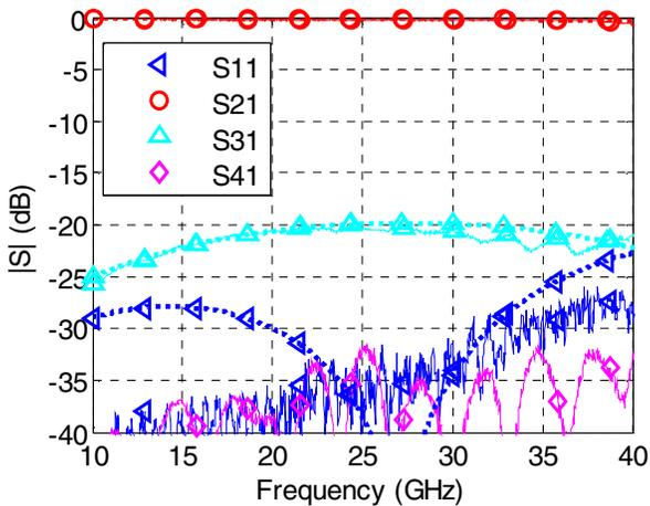
Fig. 5. Simulated (dotted) versus measured (solid) S parameters for a 20-dB coupled-line directional coupler designed for operation centered around 26 GHz.
