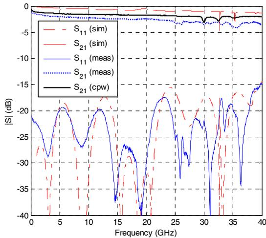
Fig. 7. A comparison of measurement and simulation for the 1-cm rectangular coaxial transmission line flip-chip attached to a CPW transition on silicon. S21 of a 11.7-mm length of CPW on silicon represents the loss from the CPW transitions to the probe pads.
