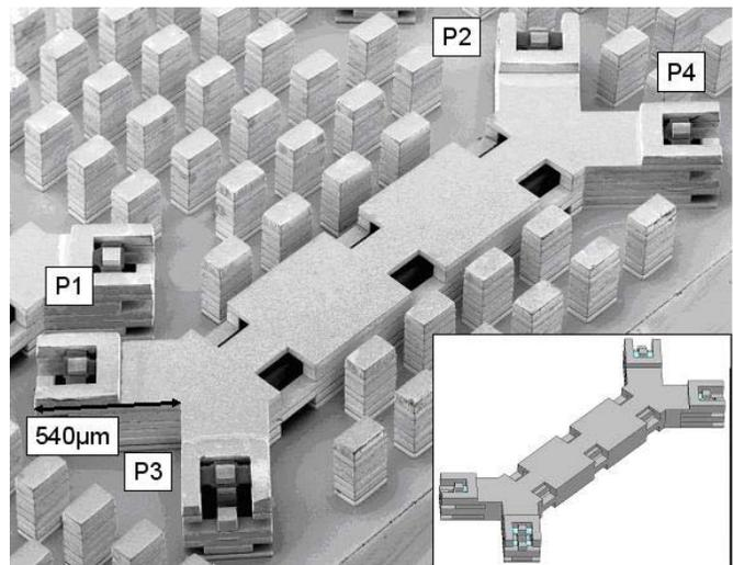
Fig. 1. An SEM image of a 10-dB directional coupler fabricated using micro-rectangular coax designed for operation centered around 26 GHz. The naming convention for the ports is labeled and an insert of the model used for simulating the design is shown in the bottom right corner.
