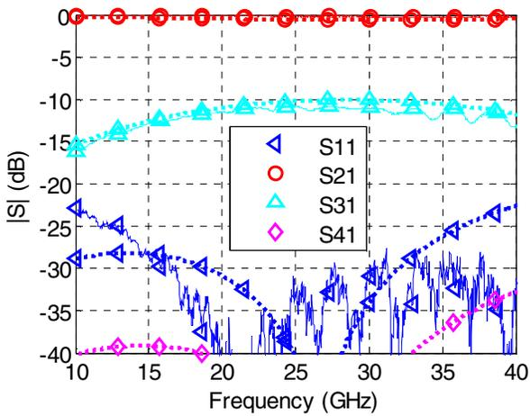
Fig. 4. Simulated (dotted) versus measured (solid) S parameters for a 10-dB coupled-line directional coupler designed for operation centered around 26 GHz.
