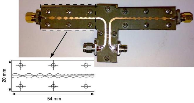
Fig. 4. Realized dispersive device. Inset: Top view of the designed CDL.
