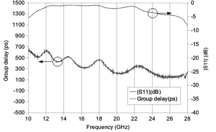
Fig. 2. Experimental measured amplitude and group delay of the reflection coefficient for the CDL realized in this work.
