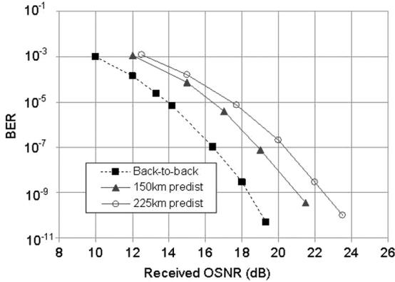
Fig. 6. Measured BER versus OSNR (resolution 0.5 nm) for different lengths of SMF propagation. Back-to-back condition with (black squares) no predistortion; (grey triangles) 150-km, and (open circles) 225-km propagation in the case of a predistorted signal.
