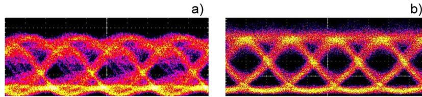
Fig. 7. Predistorted eye diagram. (a) Back-to-back and (b) after 225 km.
