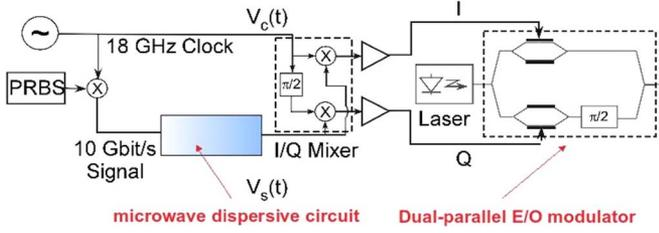
Fig. 1. Optical transmitter for analog predistortion.
