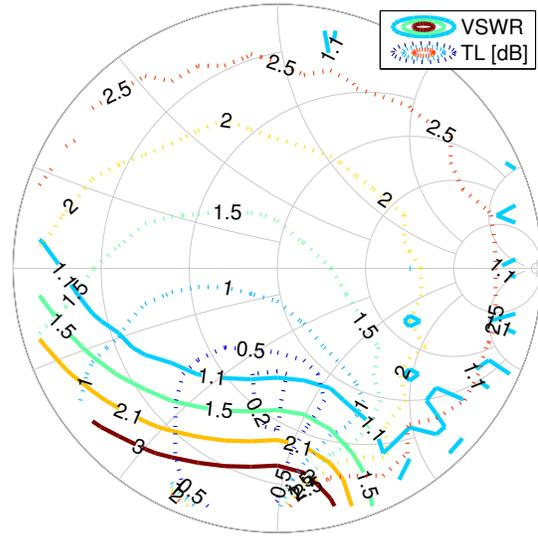
Figure 7. Measured tuner VSWR and TL at 1.95 GHz. While nearly the entire Smith chart can be reduced to VSWR of 3 or better, the insertion loss can be as high as 3 dB. Therefore, this tuner is best suited to match low-impedances that are capacitive.
