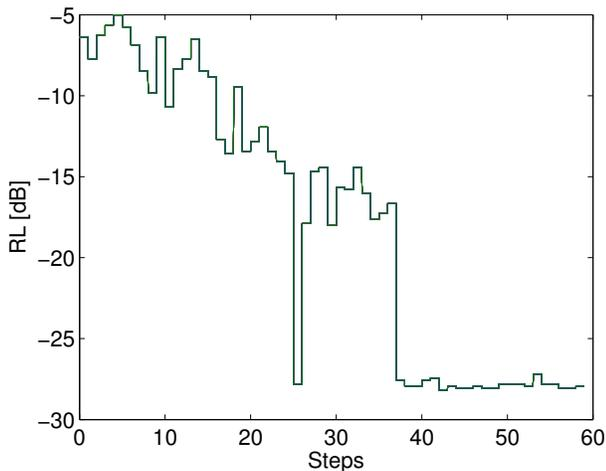
Figure 8. Measured adaptive tuner return loss convergence when the load changes from  $50\ \Omega$  to  $150\text{-}j50\ \Omega$
