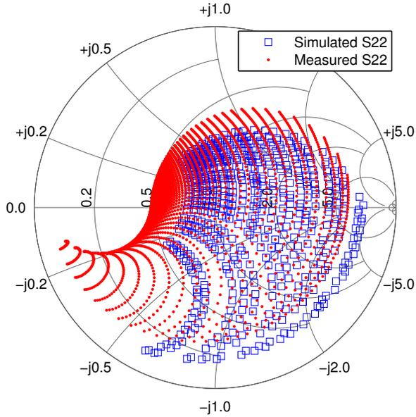
Figure 5. Simulated and measured tuner output impedance at 1.95 GHz as the reverse bias voltages are individually varied from 0 to 6.
