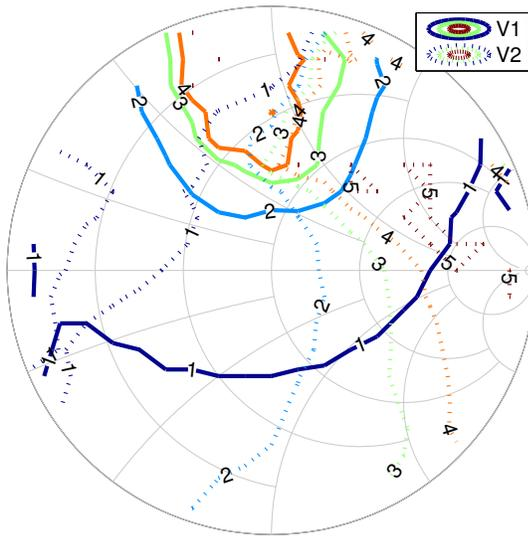
Figure 6. Measured varactor bias voltages V1 and V2 for the best match to a given load impedance at 1.95 GHz
