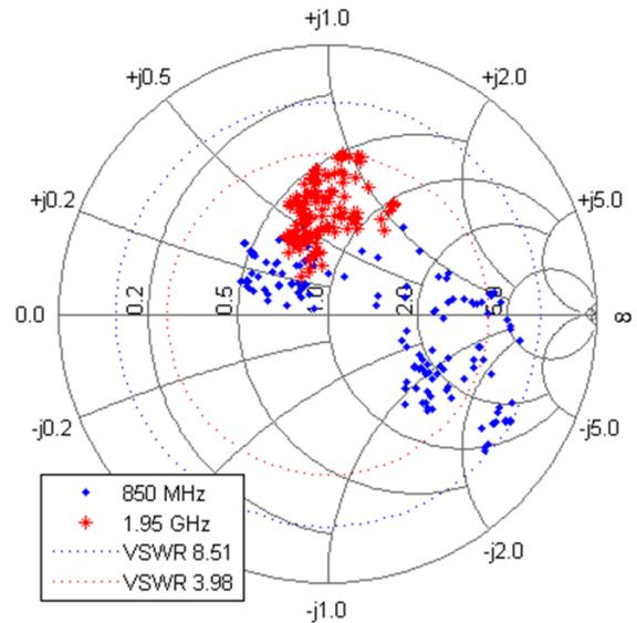
Figure 3. Measured impedance variations of a Nokia 6010 cell phone antenna under various near-field loading conditions (near head, covered by hand, on metal table, etc.).
