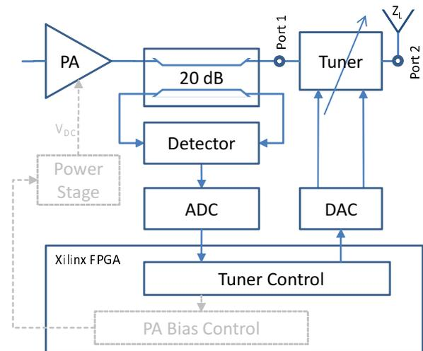
Figure 1. Block diagram of a WCDMA closed-loop tuned PA. The reflected power from a mismatched antenna is detected and digitized. The adaptive algorithm is implemented in the Xilinx FPGA and a control signal sent to both the tuner and the supply control stage.
