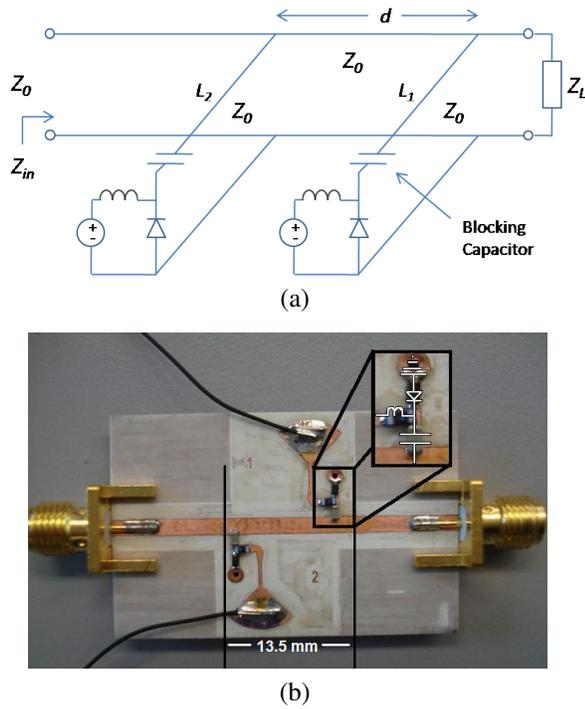
Figure 2. (a) Circuit diagram of double-stub tuner with a varactor diode at the end of the two shunt stubs and (b) a photo of the tuner circuit (13.5 mm x 23.5 mm) fabricated on 32 mil RO4003 substrate.
