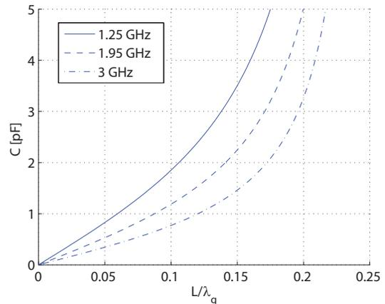
Figure 4. Equivalent capacitance of a  $50\ \Omega$  open microstrip stub vs. its electrical length. For stubs shorter than a quarter wavelength, the stubs are capacitive.
