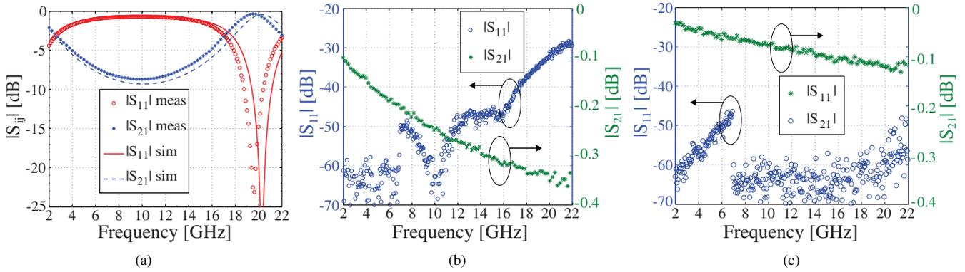
Fig. 4. (a) Simulation versus measurement results of an  $8\ \Omega$  line with  $50\ \Omega$  input and output ports. (b) Measured validation of the low-frequency TRL standard. The design frequency of this standard is 2 GHz–7 GHz. (c) Measured validation of the high-frequency TRL standard. The design frequency of this standard is 7 GHz–22 GHz.
