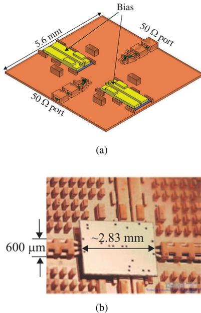
Fig. 7. (a) HFSS model of the socket, including 50 Ω input and output ports and two bias lines for gate and drain bias. (b) photograph of the active device flip-chipped to the socket. Conductive epoxy is used for electrical and mechanical connections.
