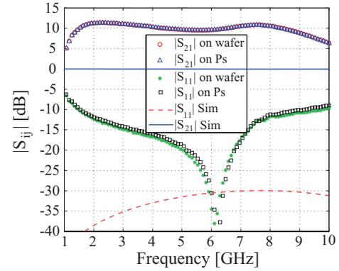
Fig. 8. Measured small-signal performance of the GaN on SiC MMIC with standard on-wafer probes compared to the performance of the same MMIC in the PolyStrata™ micro-coaxial environment. Simulation results of the socket with a 50 Ω microstrip line on a 100 μm thick SiC substrate are shown in solid and dashed lines.
