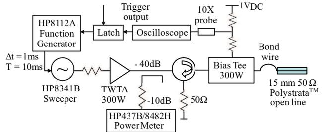
Fig. 6. Measurement setup for rf field breakdown testing performed with an open-ended  $50\ \Omega$  line with up to 300 W of input power at 10% duty cycle (1 ms duration pulses). Ionization provides a dc path through the bias tee. The detection of arcing automatically turns off the rf source, protecting the micro-coaxial line and allowing multiple tests.
