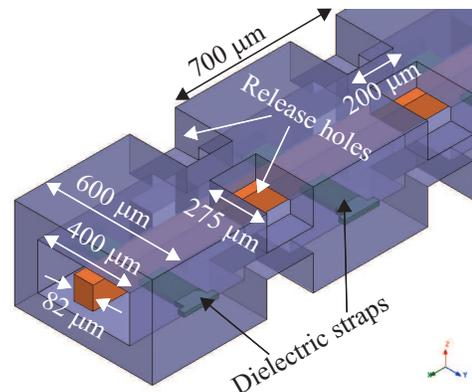
Fig. 1. Physical geometry of a 50 Ω rectangular micro-coaxial line. The inner conductor is supported in air by periodic dielectric support straps that take up a very small percentage of the total volume, resulting in very low loss [9]. The outer conductor contains holes that serve to drain the photoresist in the last fabrication step. The aspect ratio and relative dimensions of the inner and outer conductor determine the characteristic impedance.
