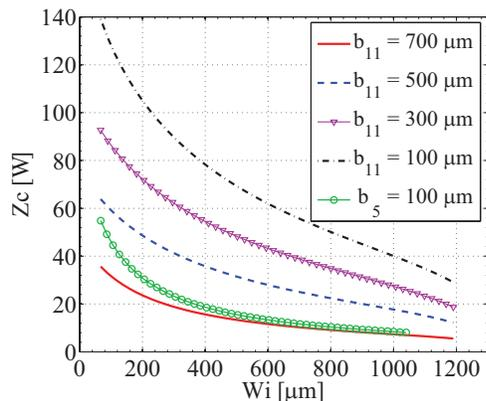
Fig. 3. Possible characteristic impedances for the eleven-layer and five-layer micro-coaxial lines versus inner conductor widths of the eleven-layer and five-layer lines. Variables  $b_{11}$  and  $b_5$  indicate the height of the inner conductor for the eleven-layer and five-layer lines, respectively. The traces labeled  $b_{11}$  correspond to  $W_a = 1350 \mu\text{m}$ , and the traces labeled  $b_5$  are for  $W_a = 1200 \mu\text{m}$ .
