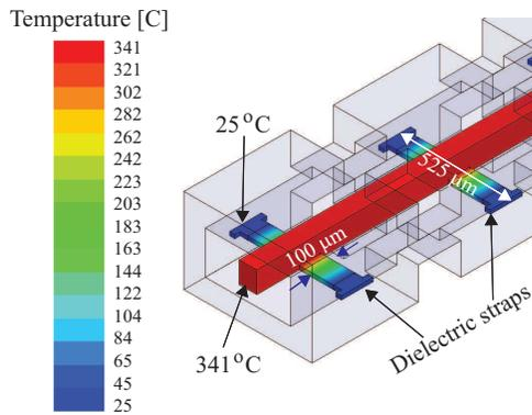
Fig. 5. This figure shows the static thermal simulation result of the five-layer low-frequency TRL line standard. The simulation is performed with Ansoft ePhysics™ for input power of 20 W. The temperature of the inner conductor increases to  $341\ ^\circ\text{C}$ , while the outer conductor temperature is kept at  $25\ ^\circ\text{C}$ .
