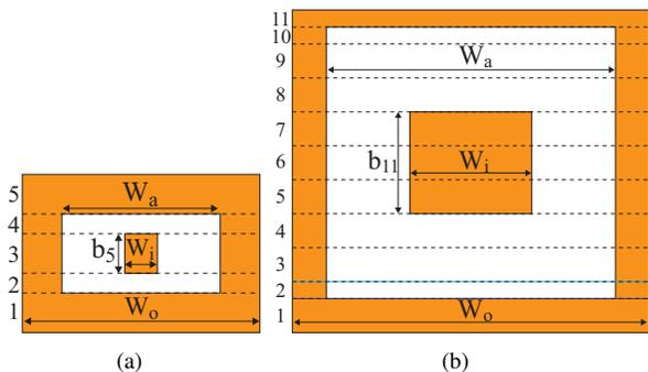
Fig. 2. (a) Cross-section of the five-layer micro-coaxial line. The height of layers 1, 3, and 5 is 100  $\mu\text{m}$ , and layers 2 and 4 are 50  $\mu\text{m}$  tall. (b) Cross-section of the eleven-layer micro-coaxial line; the height of layers 2, 10, and 11 is 50  $\mu\text{m}$ ; all other layers are 100  $\mu\text{m}$  tall.
