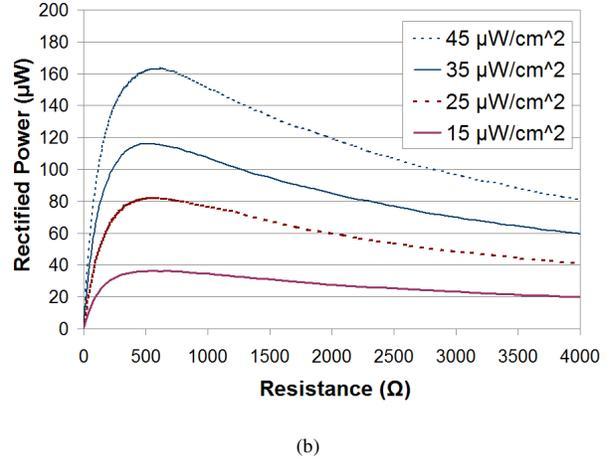
**Figure 7:** a) Image of a 6 cm x 6 cm 1.93 GHz dual-polarized patch rectenna. b) Power curves for the patch rectenna over a family of incident power densities ( $\mu\text{W}/\text{cm}^2$ ). The power curves indicate an optimal load of  $R_{em} = 500 \Omega$ . Similar power curves are measured for the other orthogonal polarization.
