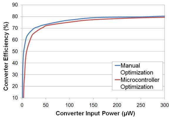
**Figure 11:** Efficiency curves of the energy harvester IC in a boost converter topology with manual and microcontroller optimization of control timing parameters,  $t_1$  and  $k$ .
