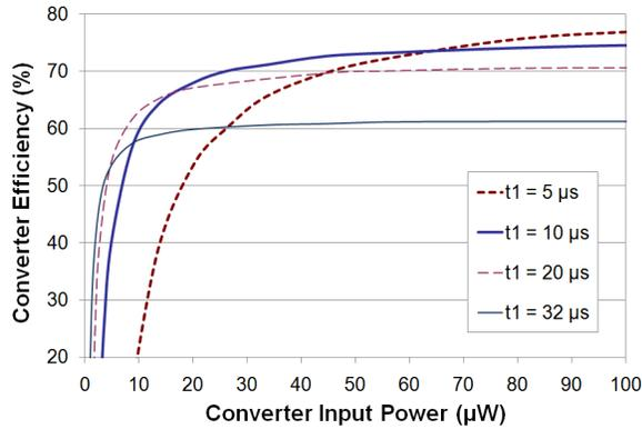
**Figure 10:** Efficiency curves of the energy harvester IC in a boost converter topology at four different control timing parameter combinations ( $t_1, k$ ). Each combination optimizes converter efficiency for four different input power levels and for  $R_{em} = 500$  .
