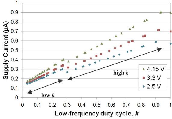
**Figure 8:** Achievable low-frequency duty cycle parameter,  $k$ , and the associated energy harvester IC supply current for three different supply voltages. The supply current includes the power consumption of the HF oscillator operating at  $t_1 = 25 \mu\text{s}$ .
