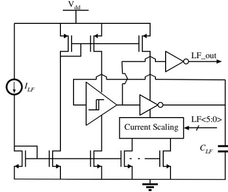
**Figure 3:** Simplified schematic of low-frequency oscillator circuitry. The current scaling block controls the current that discharges the timing capacitor,  $C_{LF}$ , and thus adjusts the  $k$  parameter.
