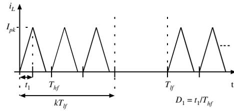
**Figure 2:** Current waveform of filter inductance,  $L$ , of a boost converter in pulsed discontinuous conduction mode (DCM). The timing parameters  $t_1$ ,  $D_1$ , and  $k$ , along with  $L$  define the converter emulated resistance,  $R_{em}$ .
