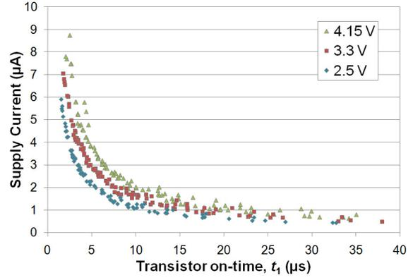
**Figure 9:** Sample of transistor on-times,  $t_1$ , that the HF oscillator can output and the associated supply current for three different supply voltages while  $k = 1$ . The full range of transistor on-times is  $0.5 \mu\text{s} < t_1 < 80 \mu\text{s}$ .
