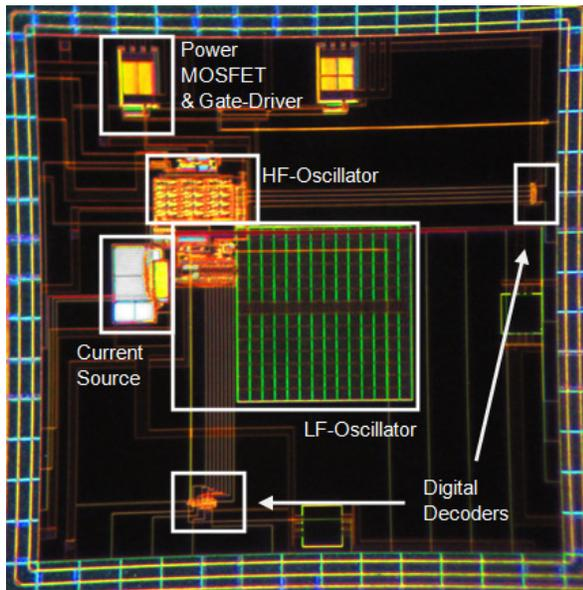
**Figure 5:** Microscope image of energy harvester IC fabricated in 5 V, 0.35  $\mu\text{m}$  CMOS process. The various circuit components are labeled. The dimensions of the chip are: 2 mm x 2 mm.
