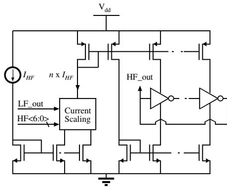
**Figure 4:** Simplified schematic of high-frequency oscillator circuitry. The current scaling block controls the current supplied into the elements of the current-starved ring oscillator and thus the  $t_1$  parameter.
