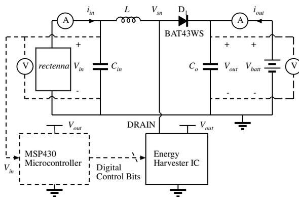
**Figure 6:** Schematic of experimental test setup for energy harvester IC used in a boost converter topology with an RF rectenna as the input power supply. The use of the IC along with an ultra-low power microcontroller is also investigated.
