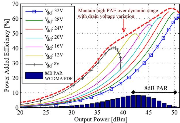
Fig. 1. Measured efficiency vs. output power for varying drain voltage for a class-AB PA prototype using a Nitronex 25100 GaN HEMT transistor. W-CDMA single-carrier down-link waveform PDF bar plot included below. The signal has been de-crested to set average power 8 dB below peak power.
