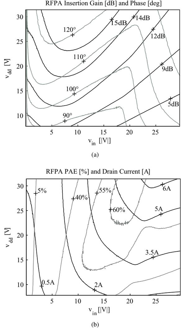
Fig. 3. Measured PA insertion gain, phase, (a), and drain current, PAE (b), over all ET operating conditions. Very low average output power (high-PAR) waveforms are used to avoid thermal interaction.
