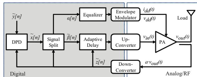
Fig. 2. One possible block diagram of an ET transmitter system.
