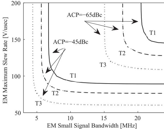
Fig. 6. EM bandwidth and slew rate required to meet -45dBc (3GPP minimum spec) and -65dBc adjacent channel power considering only distortion from the  $v_{dd}$  path for each of the signal split trajectories shown in Fig. 4(a).
