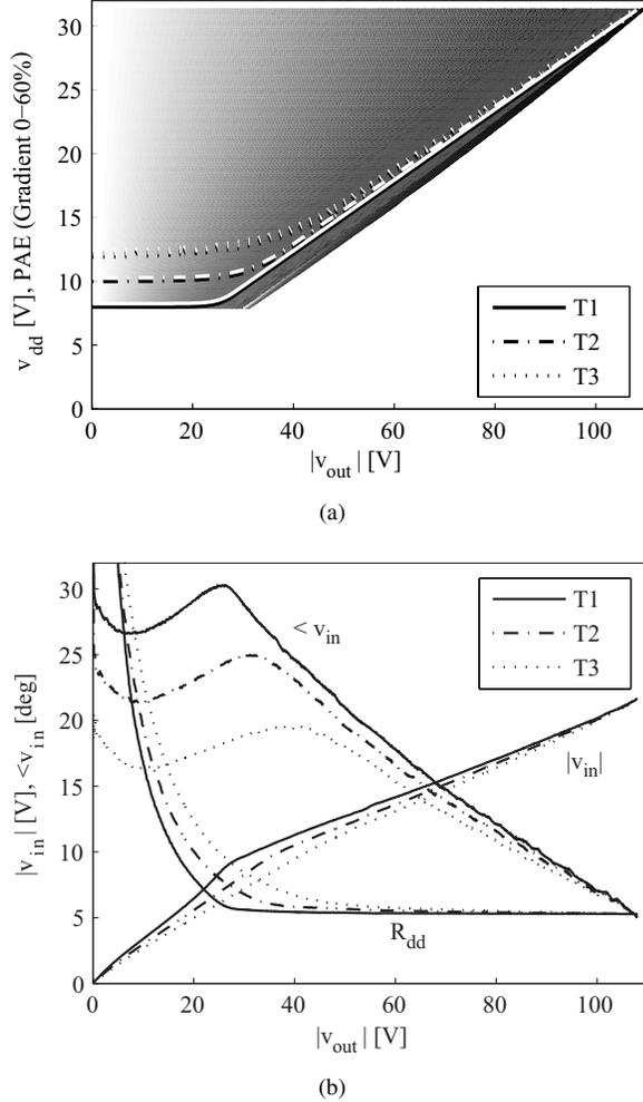
Fig. 4. (a) Three possible signal split trajectories result in varied PA modulated efficiency. The gradient indicates PA efficiency ranging from 0% to 60%. (b) PA input signal gain and phase adjustment required to account for drain voltage variation. Drain resistance is also shown at each output voltage level.
