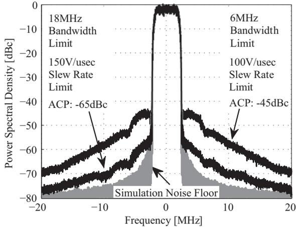
Fig. 5. Simulated ET system output power spectral density for a 1-carrier W-CDMA waveform using trajectory T2 from Fig. 4(a) given two EM models. Degradation in ACP is due only to EM non-ideality. The system noise floor shown in gray.
