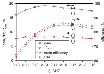
**Fig. 4** Measured gain, output power and efficiency against frequency at  $V_{DD} = 34$  V
