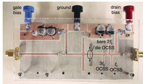
**Fig. 2** Photo of prototype amplifier measured for this Letter
