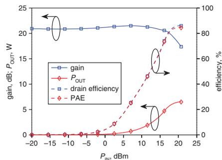
**Fig. 3** Measured PA performance at 2.14 GHz against input power,  $V_{DD} = 30$  V
