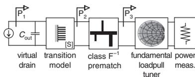
**Fig. 1** Load pull block diagram with defined reference planes for impedances
