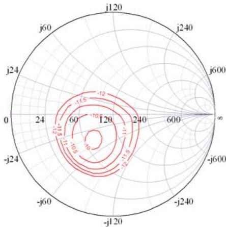
Fig. 3. Source pull contours for the Skyworks Schottky diode at 5.8GHz, showing contours of constant rectified power in dBm. The incident power is 0dBm and the DC load is 100  $\Omega$  for this measurement, and the Smith chart is normalized to 120  $\Omega$ .
