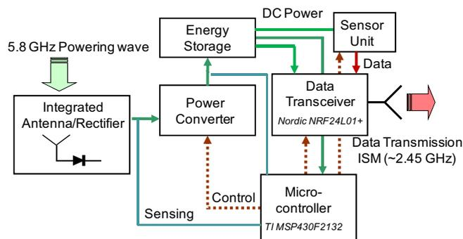
Fig. 1. Block diagram of far-field RF-powered wireless sensor. The available rectified RF power and the available energy stored are monitored (shown in light blue lines) allowing for adaptive adjustment of the data transmission duty cycle. The low-power microcontroller provides control to the power management circuit, wireless transceiver and sensor. The power is collected in the far field of one or more ISM transmitters at 5.8GHz, independently of data transmission.
