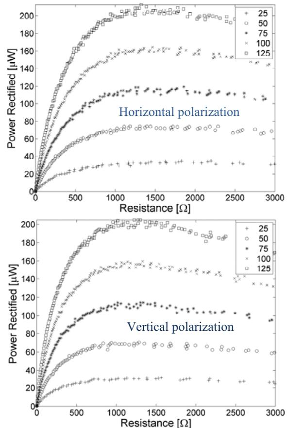
Fig. 4. Measured DC rectified power as a function of DC load for various power densities (in  $\mu\text{W}/\text{cm}^2$ ) when the normally incident wave is linearly polarized and co-polarized with each of the patch edges. The best DC load resistance is around 1000  $\Omega$  in each case and is roughly the same for the entire power range.
