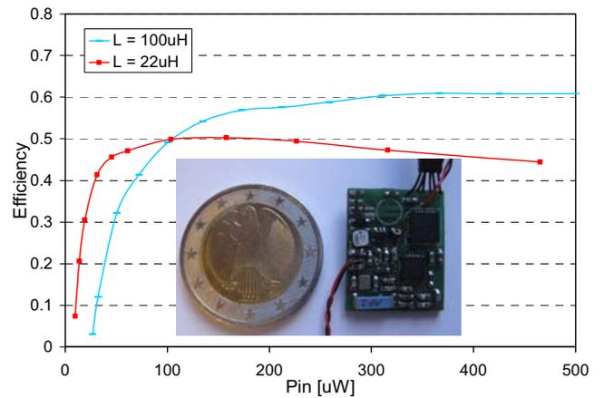
Fig. 6. Measured efficiency of circuit as a function of available input DC power for two choices of inductance value,  $L$ . The  $2.1 \times 1.7\text{cm}$  circuit contains both power management and sensor/transmitter circuitry.
