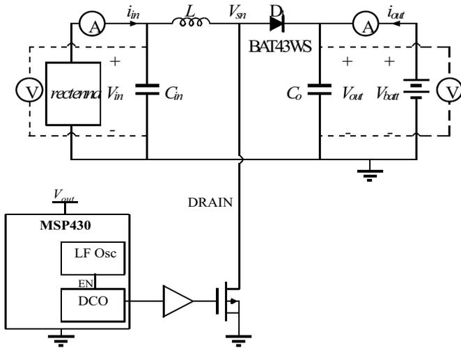
Fig. 5. Circuit diagram of the converter portion of the power management module. The rectenna is represented as an equivalent Thevenin source obtained from the measured curves in Fig. 4.
