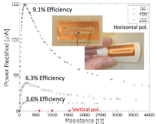
Fig. 8. Measured rectified power at 5.8GHz with a folded slot rectenna on a flexible substrate. The slot is linearly polarized and the cross-polarized rectified power is shown in red.
