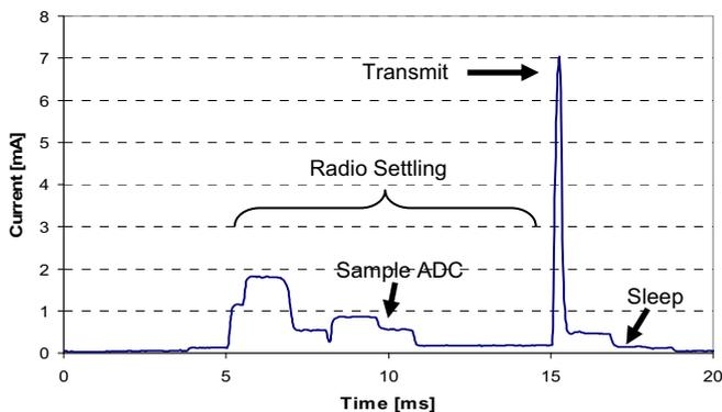
Fig. 7. Measured total current consumption of the circuit described in Fig. 1 and shown in Fig. 6.
