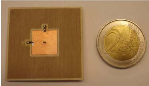
Fig. 2. Photo of integrated antenna/rectifier for 5.8GHz dual polarization reception and rectification. The antenna is fabricated on a Rogers 4350b substrate, and the diodes are soldered to the high-impedance points. The two DC connections are taken from the diode terminals and through an isolated via in the voltage null of the patch, which is 1.3mm squared in size.
