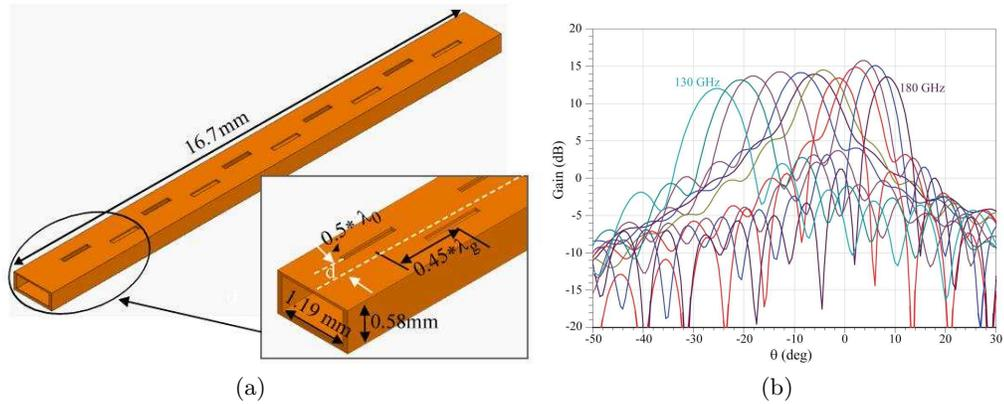
Figure 4: (a) Slotted waveguide antenna array. (b) Realized gain vs.  $\theta$  at  $\phi = 0^\circ$ , for frequencies 140–166 GHz.
