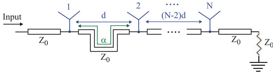
Figure 1: A conceptual sketch of an N-element frequency-scanned antenna array fed by a dispersive line.
