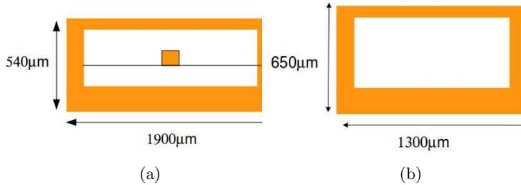
Figure 2: Typical microcoaxial (a) and waveguide (b) cross sections at G-band fabricated with the PolyStrata process.
