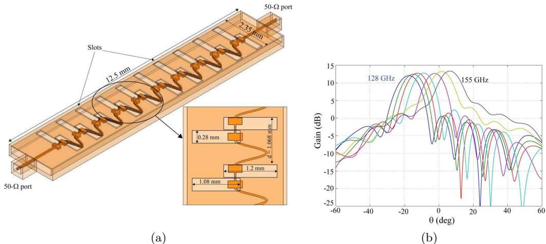
Figure 3: (a) Double slotted micro-coaxial antenna array. (b) Realized gain vs.  $\theta$  at  $\phi = 0^\circ$ , for frequencies 128–155 GHz.
