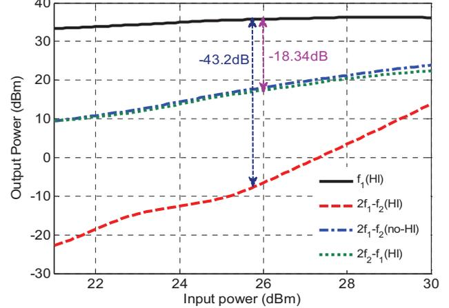
Fig. 5: Comparison of power levels for single tone and 3<sup>rd</sup> order IMD products for the HI PA and class-AB PA without harmonic injection.
