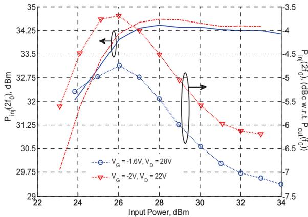
Fig. 4: Measured ratio of injected 2<sup>nd</sup> harmonic power,  $P_{inj}(2f_o)$ , to output power at the fundamental,  $P_{out}(f_o)$ , for various bias points as a function of input power at the fundamental.
