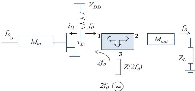
Fig. 1. Block diagram of a harmonic-injection power amplifier (HI PA) with  $2f_0$  injection at the output. A three-port network at the output allows isolation between waves at  $f_0$  and  $2f_0$  between ports 2 and 3, while allowing low loss at  $f_0$  between ports 1 and 2. The phase of the injected harmonic is critical to obtaining high efficiency.
