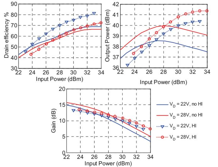
Fig. 3: Comparison of measured drain efficiency,  $P_{out}(f_0)$  and gain for the HI PA compared to the PA with no harmonic injection at  $V_D = 22\text{V}$ ,  $28\text{V}$  and  $V_G = -1.6\text{V}$  (Class A/AB).
