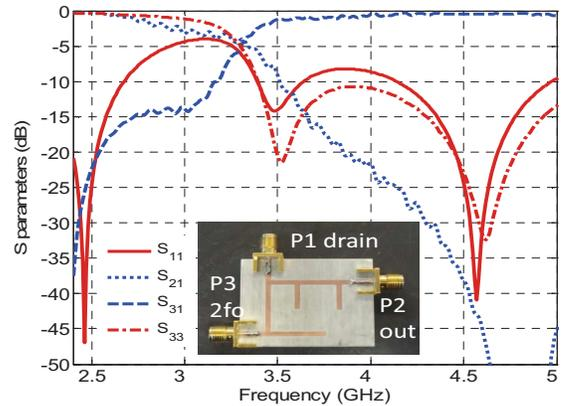
Fig. 2: Measured S parameters for the 3 port harmonic injection circuit at the output of the fundamental amplifier. A photograph of the 3 port network is shown in the inset.
