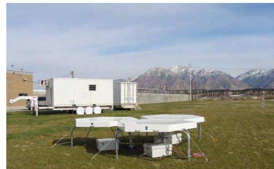
Fig. 1.(a) Block diagram of the spaced receiver 449 MHz wind profiler radar. (b) 449 MHz wind profiler deployed to the Persistent Cold Air Pool Study at Salt Lake City, Utah. Three hexagonal antennas and receivers are shown in this picture.
