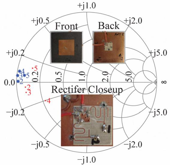
Fig. 6. Dual-linearly polarized patch rectenna and associated  $2f_0$ - $5f_0$  terminations ( $50 \Omega$  Smith Chart). Blue and red indicate the simulated and measured harmonic terminations, respectively. The rectifiers are dc isolated.
