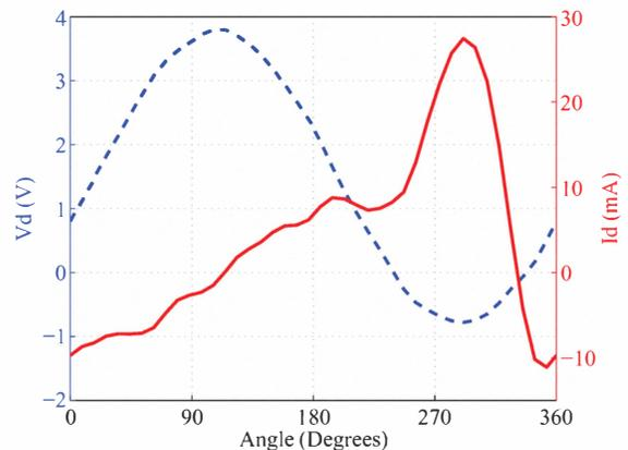
Fig. 7. Simulated time-domain current and voltage waveforms for rectifier used in dual-polarized patch antenna (using SMS7630 diode). The frequency and input power were set to 2.45 GHz and 10 dBm, respectively.
