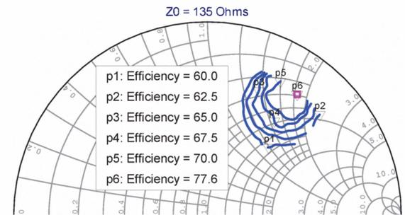
Fig. 4. Source-pull contours with available input power to the diode set to 6 dBm. The impedance is referenced to the junction capacitance of the diode, therefore the lead inductance of the package has been compensated for. Setting  $R_{DC}$  to 1080 Ω was found to result in the optimal efficiency for this input power.
