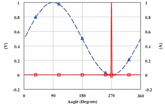
Fig. 2. Ideal normalized voltage (dashed) and current (solid) waveforms for reduced conduction angle half-wave rectifier. The waveforms have been normalized to their peak values.
