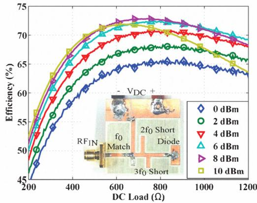
Fig. 5. RF-DC conversion efficiency versus dc load fixed available input powers with 0.6 dB matching network loss de-embedded. The maximum efficiency of 72.8% occurred at 8 dBm with  $R_{DC} = 742 \Omega$ , which is lower than the  $1080 \Omega$  found during source-pull. However, the efficiency at  $1080 \Omega$  is 69.9% which is very close to the peak value.
