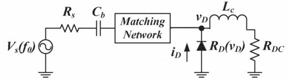
Fig. 1. Microwave rectifier circuit diagram. An ideal blocking capacitor  $C_b$  provides dc isolation between the microwave source and rectifying element. An ideal choke inductor  $L_c$  isolates the dc load  $R_{DC}$  from RF power.
