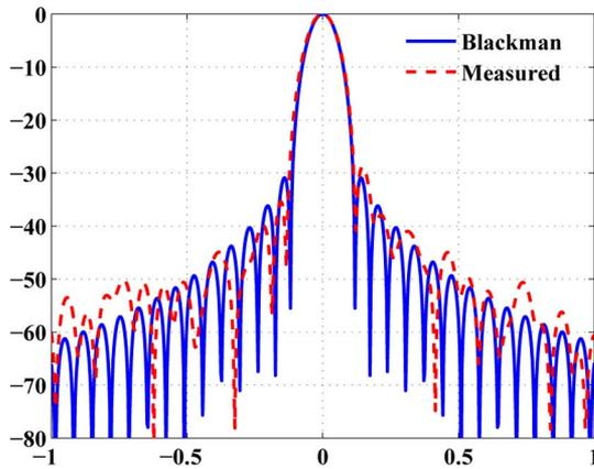
Fig. 6. Normalized frequency response of the measured power spectrum. The is consistent with the frequency response resultant from shaping the power using a Blackman power window, which is shown in the solid blue curve.
