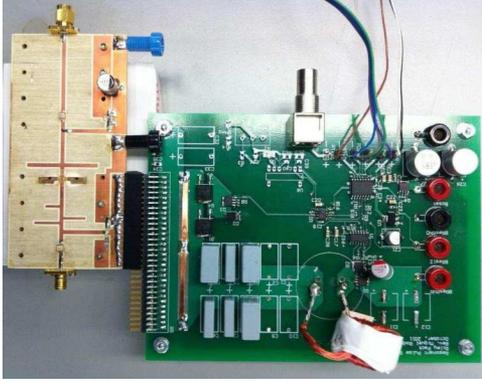
Fig. 2. Photo of the amplifier integrated with the pulsing circuit.
