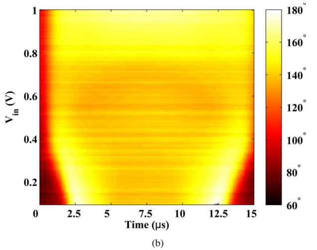
Fig. 5. (a) Gain magnitude variation as a function of input voltage and time, normalized to peak input voltage. (b) Gain phase variation as a function of input voltage and time, normalized to peak input voltage.
