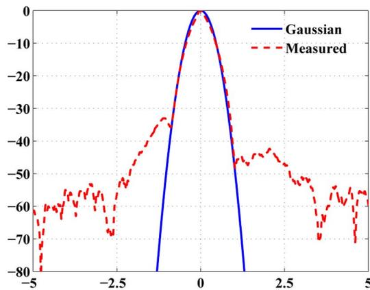
Fig. 7. Normalized frequency response of the measured power spectrum. The is consistent with the frequency response resultant from shaping the power using a 12 dB Gaussian power window, which is shown in the solid blue curve.
