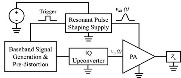
Fig. 1. Block diagram of radar transmitter with resonant pulse shaping supply for shaping the waveform envelope allowing spectral confinement of the transmitted waveform.
