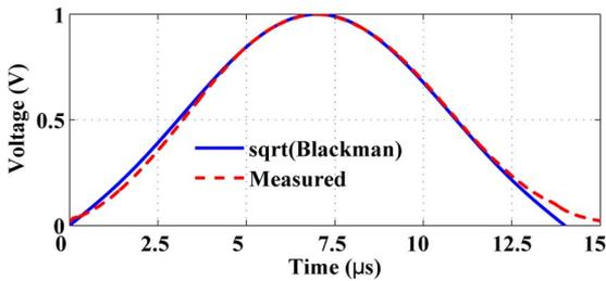
Fig. 4. Measured supply voltage versus time. The measured supply voltage is well approximated by the square root of a Blackman windowing function.
