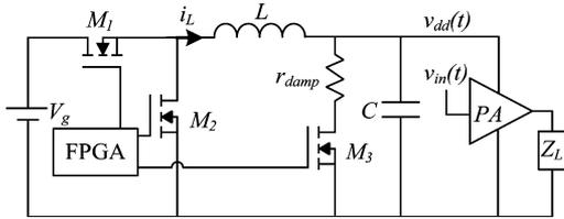
Fig. 3. Block diagram of resonant pulse shaping supply implementation.
