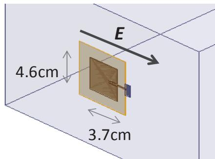
Fig. 3. Geometry of patch probe 1 from Fig.1 placed on the inside wall of the resonator, with the patch ground plane connected to the cavity walls. The microstrip radiating-edge indented feed is connected to the power transmitter which is external to the cavity. The second probe from Fig.1 is orthogonally-polarized relative to probe 1.
