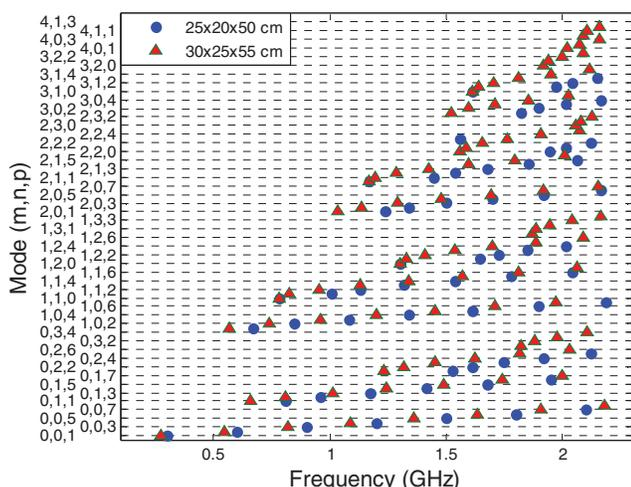
Fig. 8. TE and TM mode cutoff frequencies calculated for a 20cmx25cmx50cm and a 25cmx30cmx55cm rectangular resonator. The number of modes and spectral distribution increase when the cavity is enlarged by a third of a wavelength at 2.2GHz.
