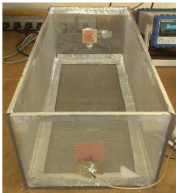
Fig. 7. Assembled prototype powering cavity with two probe feeds oriented orthogonally to each other. The metal screening is used as a reflector that keeps all radiation within the box while the lid is closed but enables visual inspection.
