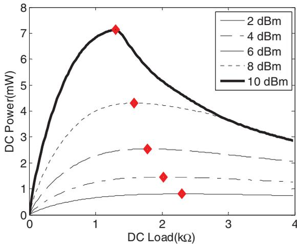
Fig. 5. Simulated load-pull plot of rectifier with RF input of varying power levels, with diamond markers indicating the optimal load resistance for maximum rectified power at each input power level. Note that the optimal load point varies with input power.
