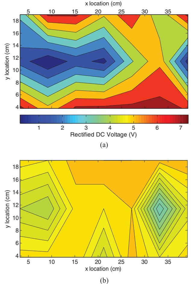
Fig. 6. Measured DC voltage rectified from receive probe placed at varying locations throughout the cavity, oriented such that its radiating edge is perpendicular to the radiating walls ( $x = 0$  cm,  $50$  cm). The probe did not vary in any other dimension, resting on a 24 mm thick polystyrene shelf. The rectifier was loaded with a 1.5-kΩ resistor (a) and an active load with MPPT (b). The excitation probes remained fixed at  $y = 12.5$  cm and  $x \approx 0$  cm,  $50$  cm.
