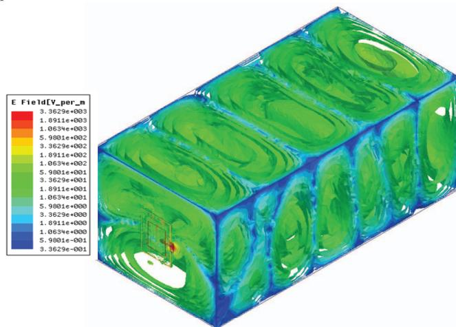
Fig. 4. Simulated electric field profile in the unloaded resonator when excited with the two patch probes fed 135 degrees out of phase. The sources are not modulated, resulting in a non-uniform field distribution.
