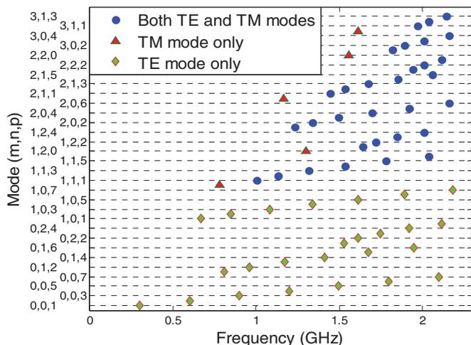
Fig. 2.  $TE_{mnp}$  and  $TM_{mnp}$  mode cutoff frequencies calculated for a rectangular metallic resonator 20cm x 20cm x 50cm in size.
