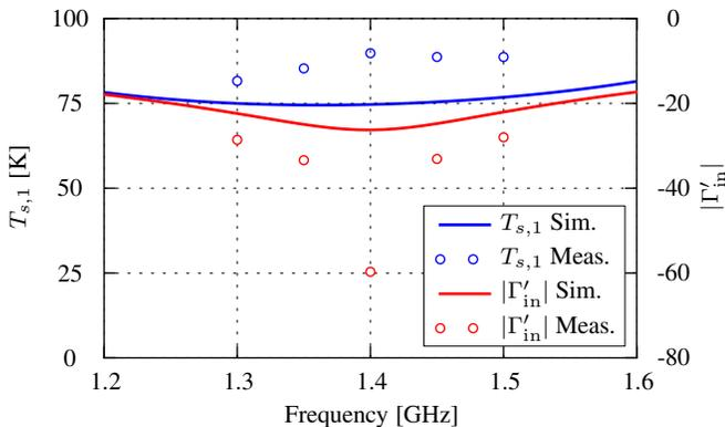
Fig. 9. Measured  $T_{s,1}$  and reflection coefficient of the packaged MMIC noise source demonstrating an equivalent noise temperature of approximately 90 K while maintaining an input reflection coefficient of less than -50 dB at 1.4 GHz.
