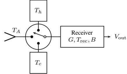
Fig. 1. Block diagram for a radiometer demonstrating calibration with hot ( $T_h$ ) and cold ( $T_c$ ) calibration standards.
