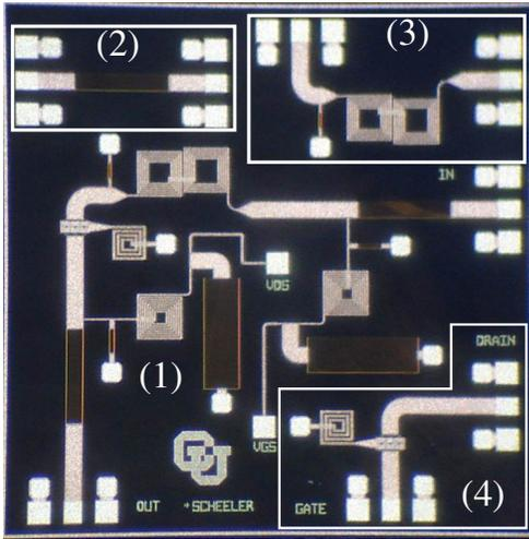
Fig. 8. Photo of the 1.4 GHz GaAs MMIC. The noise source with the input and output bias tees and input matching network is labeled by (1). The test circuits are a blocking capacitor (2), input matching network (3), and transistor test circuit (4).
