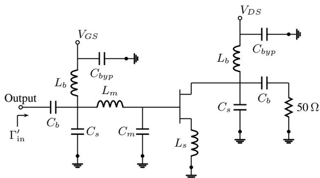
Fig. 5. Schematic of the active cold noise source. Additional source inductance was added such that the optimum load impedance is  $50\ \Omega$  such that no output matching network is needed.
