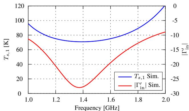
Fig. 7. Simulated  $T_{s,1}$  and input match of the MMIC ACL demonstrating a  $T_{s,1} = 70.9\text{ K}$  with an input match of  $-27\text{ dB}$  at 1.4 GHz.
