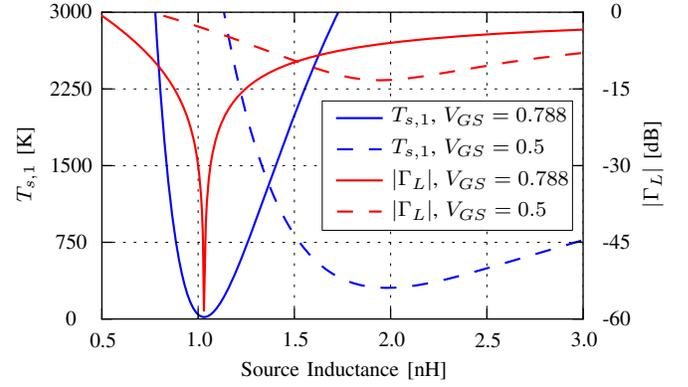
Fig. 3. Simulated  $T_{s,1}$  and  $|\Gamma_L|$  calculated from (5) for a TriQuint  $0.5 \mu\text{m}$  pHEMT device. The transistor was biased at  $1.7 \text{ V}$  on the drain and the ideal source inductance was varied from  $0.5 \text{ nH}$  to  $3 \text{ nH}$  for two different gate biases corresponding to  $0.5 \text{ V}$  and  $0.788 \text{ V}$ . A minimum in  $T_{s,1}$  is achieved when  $|\Gamma_L|$  is minimized.
