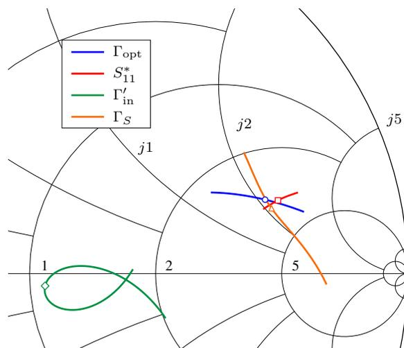
Fig. 6. Simulated optimum noise match and the conjugate of the reflection coefficient looking into the device are shown along with the reflection coefficient looking towards the source ( $\Gamma_S$ ) through the input match and bias network vs. frequency from 1 to 2 GHz. The input match is shown looking into the noise source ( $\Gamma'_{in}$ ). The Smith chart is normalized to  $50\ \Omega$ , and the markers on the plot correspond to 1.4 GHz.
