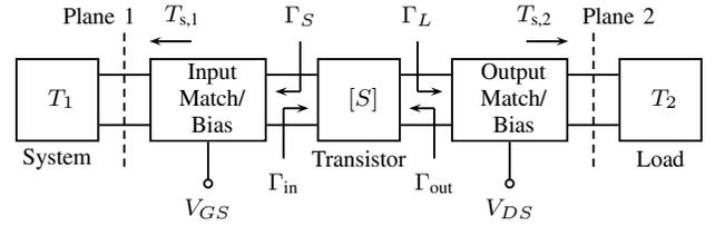
Fig. 2. Block diagram for the ACL design showing the input and output matching and bias networks necessary for the design in which the input of the device is presented with  $\Gamma_S$  and the output of the device is presented with  $\Gamma_L$ .
