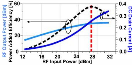
Fig. 6. Circuit-B as an amplifier: PAE (black dashed line), output RF power (light blue) and DC drain current (dark blue) versus input RF power. The best efficiency is  $PAE = 56.47\%$  at  $P_{in} = 26$  dBm (red dashed line) with  $V_{GG} = -3.4$  V,  $V_{DD} = 20$  V.
