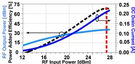
Fig. 3. Circuit-A best efficiency performance as an amplifier is measured with  $V_{GG} = -4.0$  V and  $V_{DD} = 20$  V. Light blue curve is the output power, dark blue is the DC drain current and the efficiency ( $PAE$ ) is traced with a black dashed line. The maximum efficiency is  $PAE = 67.87\%$  at  $P_{in} = 26.42$  dBm (red dashed line).
