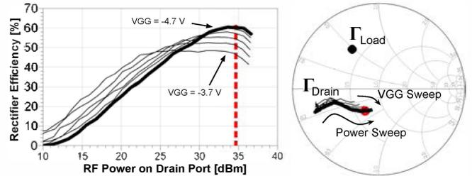
Fig. 4. Circuit-A rectifying performance for  $V_{GG}$  between  $-3.7$  V and  $-4.7$  V with a 0.2 V step. The gate RF port is terminated at the fundamental frequency with  $Z_{load} = (17.9 + j 24.0)\Omega$  and the drain DC load impedance is  $R_D = 100\Omega$ .
