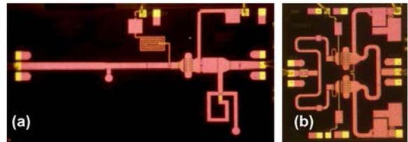
Fig. 1. X-Band MMIC power amplifiers operated as rectifiers. (a) Circuit-A: single-stage single-ended PA, using a  $10 \times 100\mu\text{m}$  transistor. The die is  $3.8 \times 2.3\text{mm}^2$  in size. (b) Circuit-B: single-stage power combined PA, with two  $10 \times 100\mu\text{m}$  transistors, and an overall footprint of  $2.0 \times 2.3\text{mm}^2$ .
