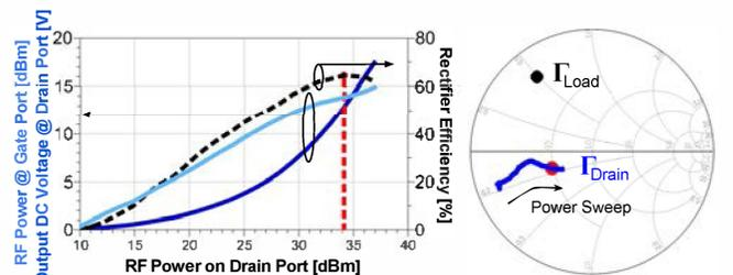
Fig. 5. Circuit-A: Rectifier efficiency  $\eta_R$  (black dashed line), DC output drain voltage (dark blue) and RF power at the gate reference plane (light blue) versus injected drain RF power. The best rectifying performance is  $\eta_R = 64.4\%$  at  $P_{RF} = 34.14$  dBm (red dashed line). The Smith chart on the right shows the optimal load impedance presented at the gate port (black dot) and the drain impedance of the DUT (blue curve) during the power sweep.
