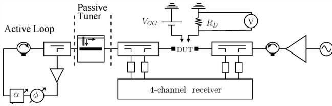
Fig. 2. Time-domain measurement setup for rectifier characterization. A load-pull is performed at the gate RF port of the DUT, with a passive tuner and an active loop that enables a highly reflective load impedance at 10.1 GHz.
