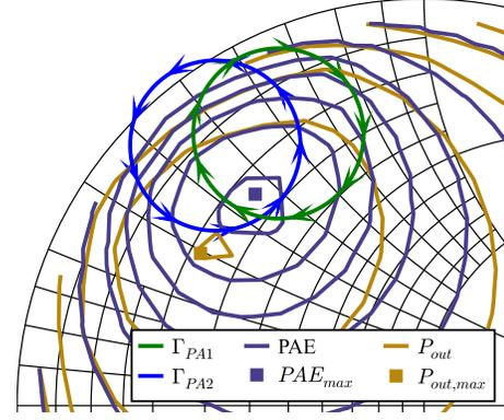
Fig. 3. Load modulation of each PA,  $\Gamma_{PA1}$  and  $\Gamma_{PA2}$ , overlaid on PAE and  $P_{out}$  load-pull contours, at combiner reference plane.
