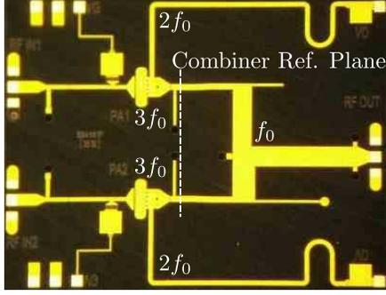
Fig. 2. Photograph of ML-CO GaN MMIC PA, showing harmonic terminations and combiner design reference plane. The internal PAs operate in Class-F, with the combiner providing all fundamental frequency matching. Overall size is 3.8 mm  $\times$  3.2 mm.
