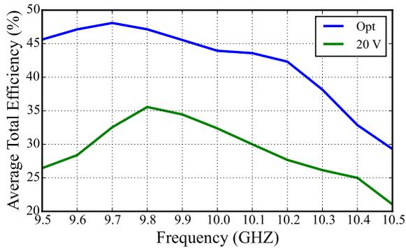
Fig. 9. Comparison of average total efficiency across frequency between the optimal trajectory and 20 V supply, showing improvements between 8 and 19 points. Optimal operation achieves 400 MHz of bandwidth with  $\eta_{tot,avg} > 45\%$ .
