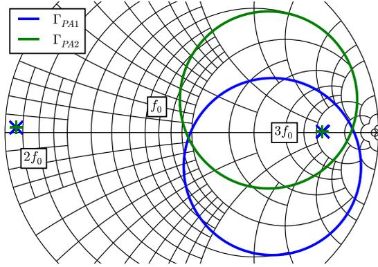
Fig. 5. Simulated load modulation at the intrinsic drain of each PA during outphasing. The high Q of the resonators used in the harmonic terminations keeps their impedances from changing even as the fundamental load modulates. The effectiveness of the  $3f_0$  termination reduces as the fundamental load becomes larger than it with increasing outphasing angle.
