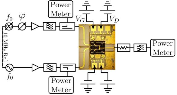
Fig. 7. ML-CO measurement setup. Separate sources drive each PA branch, while a phase shifter sweeps the differential phase. The source driving the phase shifter adjusts its amplitude to maintain constant available input power to within 0.1 dB.
