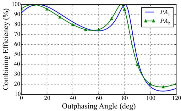
Fig. 6. Simulated combining efficiency of the microstrip combiner (referenced to the intrinsic drain) is maintained above 70% over 85° of outphasing range.
