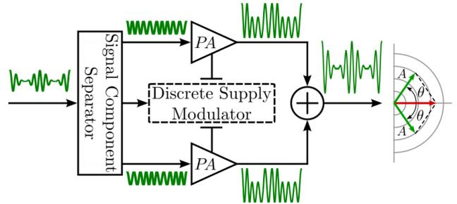
Fig. 1. Block diagram of Multi-Level Chireix Outphasing, showing the signal component separation, which must control the additional phase modulation ( $\theta$ ) as well as amplitude control via the discrete supply modulator. The combiner is a lossless, three-port network, often incorporating Chireix compensation.
