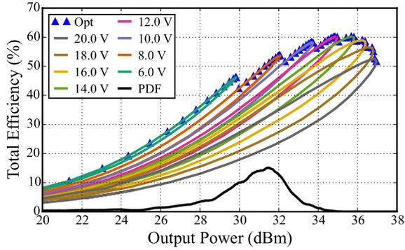
Fig. 8. Compilation of measured phase sweeps for swept supply levels from 6 V to 20 V in 2 V increments at 9.7 GHz. The optimal trajectory is selected to maximize  $\eta_{tot}$ . In black is the PDF of a 6 dB PAPR QPSK signal used to calculate average total efficiency.
