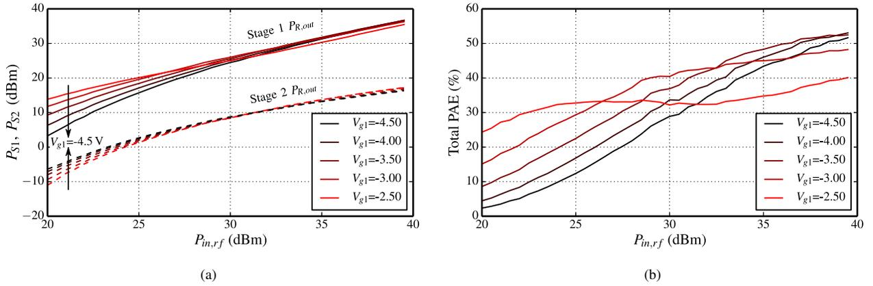
Fig. 3: (a) Stage 1 and Stage 2 rectified power as a function of RF input power at various Stage 1 gate bias voltages ( $V_{G1}$ ). (b) Total RF-DC conversion efficiency. The optimal bias point depends on input power. For high input power, a lower gate bias for Stage 1 and a higher gate bias for Stage 2 gives maximum output power for each stage respectively. The measurement is performed at 9.9 GHz with  $R_{DC1} = R_{DC2} = 30 \Omega$ .
