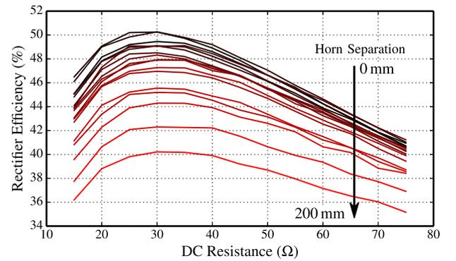
Fig. 4: Stage 1 DC rectified efficiency (RF to DC) versus DC load and increasing horn separation. The optimum DC load resistance is approximately  $30 \Omega$  regardless of the input power. The input power versus horn separation is shown in Fig. 6a.
