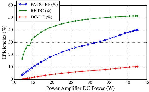
Fig. 5: Wireless link efficiencies of the power amplifier, rectifier, and total system efficiency versus total DC power consumed in watts. Peak system efficiency of  $>10\%$  is achieved with the highest DC power consumed by the PA.
