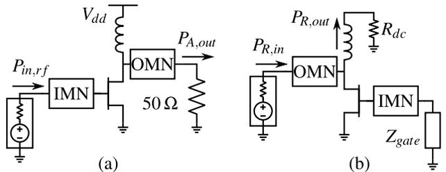
Fig. 1: (a) Block diagram of PA with a FET transistor. (b) Block diagram of PA used as a rectifier.
