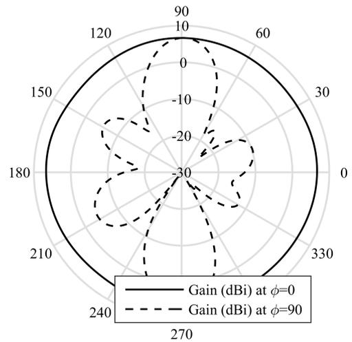
Fig. 3. Simulated gain of the air-substrate CoCo antenna as a function of  $\theta$ , for  $\phi = 0^\circ$  (solid line) and  $\phi = 90^\circ$  (dashed line) along with the simulated gain of the air-substrate CoCo antenna for  $\phi = 0^\circ$  (dotted line) and  $\phi = 90^\circ$  (dash-dot line) at frequency of 2.45 GHz.
