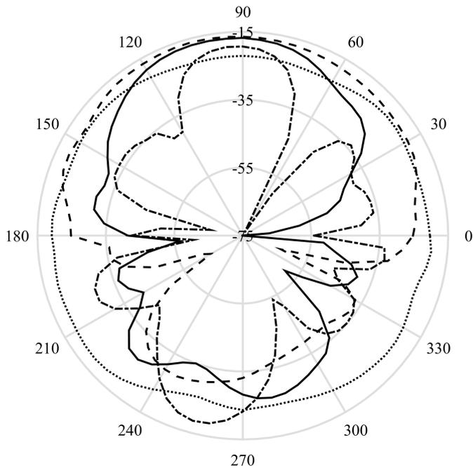
Fig. 6. Measured harvested power of the patch rectenna (dBm) as a function of  $\theta$  at the incident power density of  $1 \mu\text{W}/\text{cm}^2$ , for  $\phi = 0^\circ$  (solid line) and  $\phi = 90^\circ$  (dashed line) along with the measured harvested power of the CoCo rectenna for  $\phi = 0^\circ$  (dotted line) and  $\phi = 90^\circ$  (dash-dot line) at frequency of 2.45 GHz.
