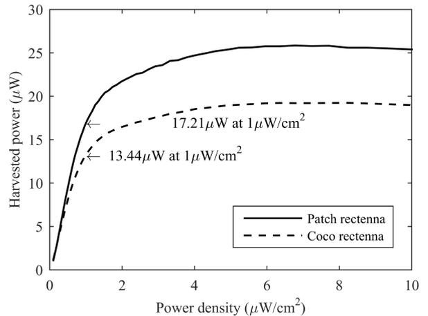
Fig. 5. Measured harvested power of the patch and CoCo rectennas as a function of power density. At the power density of 1 the harvested power for the patch and CoCo rectennas are 17.21 and 13.44  $\mu\text{W}$ , respectively.
