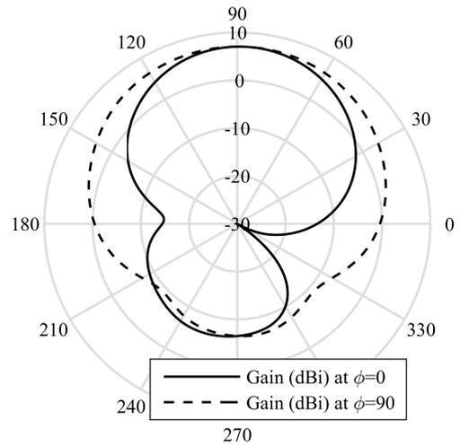
Fig. 2. Simulated gain of the air-substrate patch antenna as a function of  $\theta$ , for  $\phi = 0^\circ$  (solid line) and  $\phi = 90^\circ$  (dashed line) along with the simulated gain of the air-substrate CoCo antenna for  $\phi = 0^\circ$  (dotted line) and  $\phi = 90^\circ$  (dash-dot line) at frequency of 2.45 GHz.
