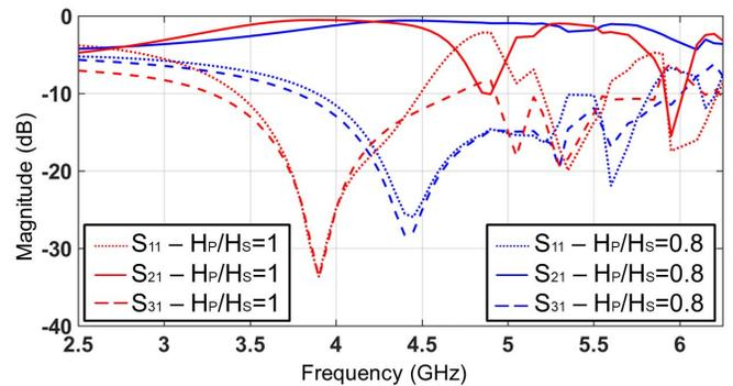
Fig. 2. Electromagnetically-simulated response in terms of S-parameters for alternative levels of  $H_P/H_S$ . The circulator dimensions and the applied DC magnetic bias field are identical for both designs.
