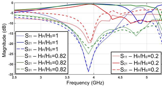
Fig. 3. Electromagnetically-simulated response in terms of S-parameters for alternative levels of  $H_p/H_s$ . The circulator dimensions are identical for both designs. The DC magnetic bias field is altered as shown in Fig. 4.
