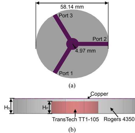
Fig. 1. (a) Top view. (b) Cross-sectional view of the microstrip-line type circulator. The material properties are summarized as follows: Dielectric substrate: Rogers 4350,  $\epsilon_r=3.66$ ,  $H_S=1.524$  mm, Ferrite puck: TransTech TT1-105:  $M_S=0.175$  T,  $\epsilon_r=12.2$ ,  $\mu_0=55$ ,  $\Delta H=220$  Oe,  $H_P \leq 1.524$  mm. The conceptual drawings of the circulator are not in scale.
