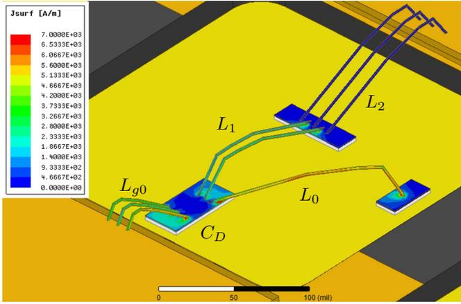
Fig. 3. HFSS model of the passive-only in-packaged matching circuit showing a plot of  $2f_0$  of surface current magnitude along the bond wires and on the capacitor plates. The current along  $L_0$  is pronounced (600 A/m), since it is responsible for the  $2f_0$  drain termination. Notice that there is more current on the bond-wire closest to  $L_0$  than the other bond-wire at that point in the network. This is due to mutual inductance.
