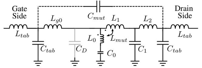
Fig. 4. Equivalent circuit model of passive package shown in Fig. 1b. The active device in Fig. 1a is replaced by a capacitor  $C_D$  of similar size and known value, represented by capacitor  $C_D$  in grey.
