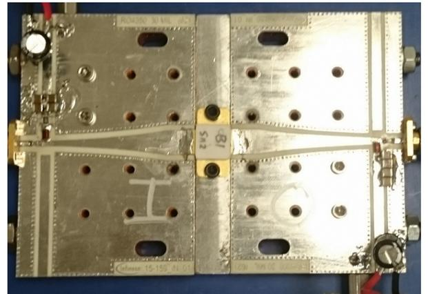
Fig. 5. Microstrip fixture used for TRL calibration and measurement of the validation package. The package is mounted on a 280-mil wide microstrip line and tapered to a  $50\Omega$  environment. Bias-tees are integrated into the fixture anticipating large-signal measurements with the active package but are not necessary for the validation process.
