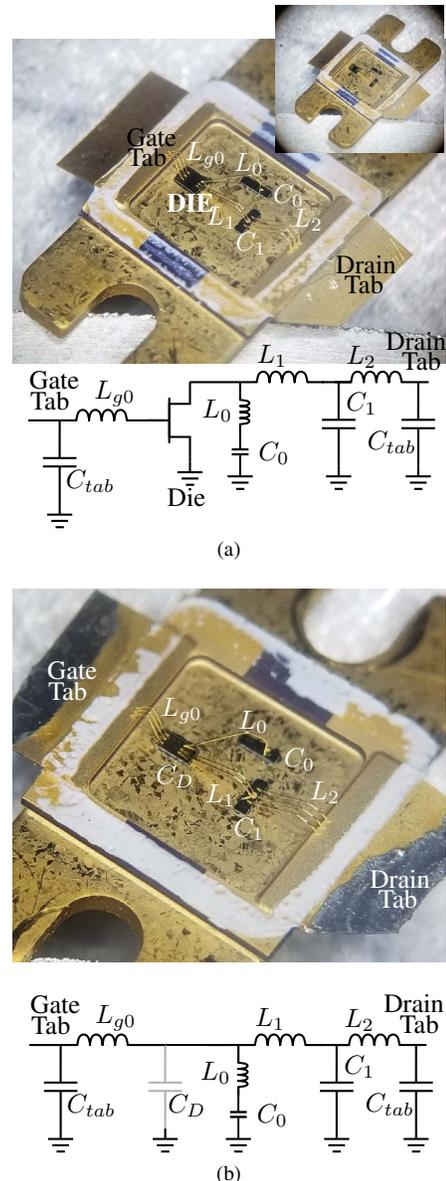
Fig. 1. (a) Transistor package for an Infineon 10-W LDMOS device with a fundamental of 2.6 GHz. The package is custom designed for a fundamental pre-match and a 2<sup>nd</sup> harmonic termination both internal to the package. (b) Passive validation package, where the active device is replaced by a capacitor of similar size and known value. Circuit diagrams are also shown, where the inductors represent bond-wires and the drain and gate tabs are represented by capacitors.
