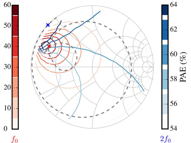
Fig. 2. Loadpull contours for constant PAE for varied fundamental (red scale) and  $2^{nd}$  harmonic (blue scale) load impedance. The impedance presented to the device drain terminal by the in-package passive circuit from Fig. 1 over the 1 to 8 GHz frequency range is shown by the dashed gray trace, with the  $f_0$  and  $2f_0$  impedances indicated by the red and blue crosses, respectively.
