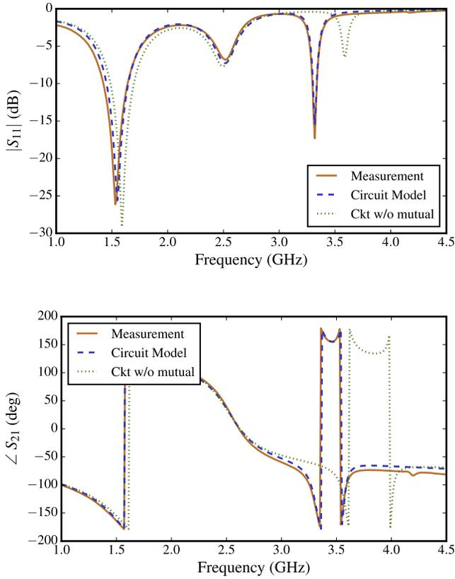
Fig. 6. Measured (solid line) vs. simulated (dashed line)  $S$ -parameters of the equivalent package circuit model from Fig.4. The elements  $C_{mut}$  and  $L_{mut}$  are omitted from this circuit model and also plotted (dotted line) to illustrate the distinct impact of these values on the impedance presented to the packaged device.
