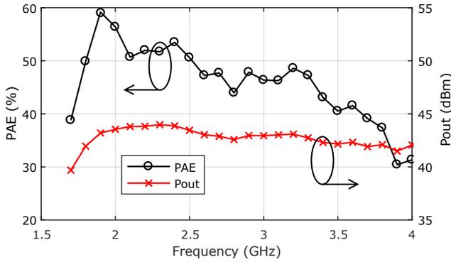
Fig. 2. Measured (CW) maximum  $PAE$  and  $P_{OUT}$  of the RF-input LMBA with fixed bias between 1.7 to 4 GHz [6].
