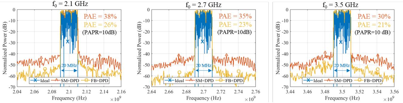
Fig. 6. Measured output spectra of the ET-LMBA at 2.1, 2.7 and 3.5 GHz for a 20-MHz, 10-dB PAPR signal. Supply modulation (SM) and fixed bias (FB) operation are compared, both with DPD.
