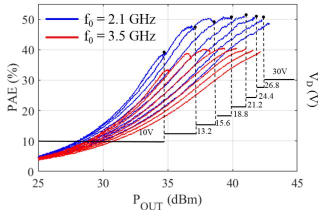
Fig. 5. PAE characteristics of the ET-LMBA at the eight voltage levels and at two carrier frequencies at the band edges, 2.1 and 3.5 GHz. The discretized supply shaping table for 2.1-GHz also shown.
