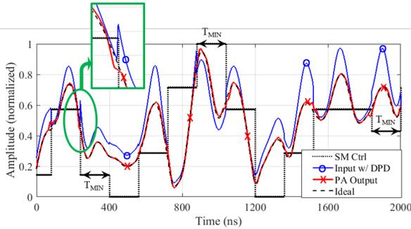
Fig. 7. Measured output envelope of the ET-LMBA for a 20-MHz, 10-dB PAPR signal at 2.1 GHz. The DPD successfully linearizes the ET-LMBA behavior at multiple supply levels.
