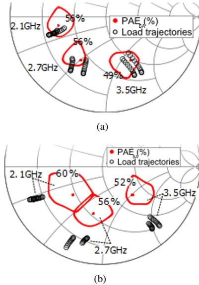
Fig. 3. Simulated PAE and load trajectories at 2.1, 2.7 and 3.5 GHz. (a) Simulated PAE at  $v_D = 30$  V. (b) Simulated PAE at  $V_D = 15$  V. The control PA supply voltage is held constant at 20 V.
