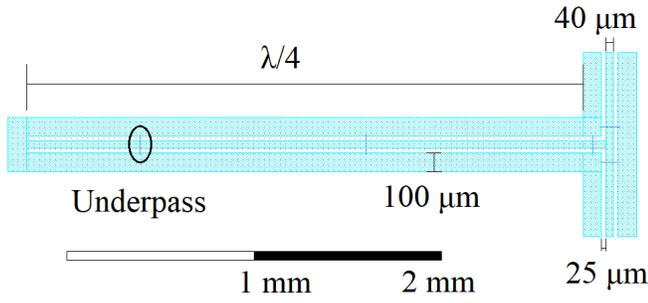
Fig. 2. ADS layout of a 50-Ω CPW line with  $\lambda/4$  shunt shorted stub and  $\lambda/10$  spaced underpasses, currently in fabrication. Labeled line width, gap width, and ground width are the same everywhere in this layout.
