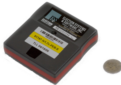
Figure 2: An ES&S “Personalized Electronic Ballot” (PEB) used to transport ballots and results between the iVotronic and Unity.
