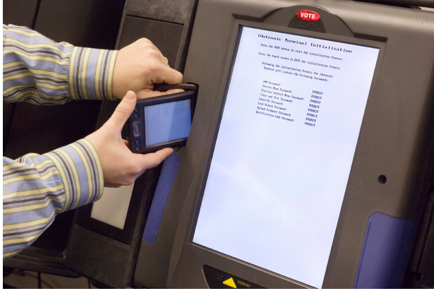
Figure 3: A PEB emulator running on a Palm device simulates an initialization PEB during an open election, resetting all iVotronic passwords.
