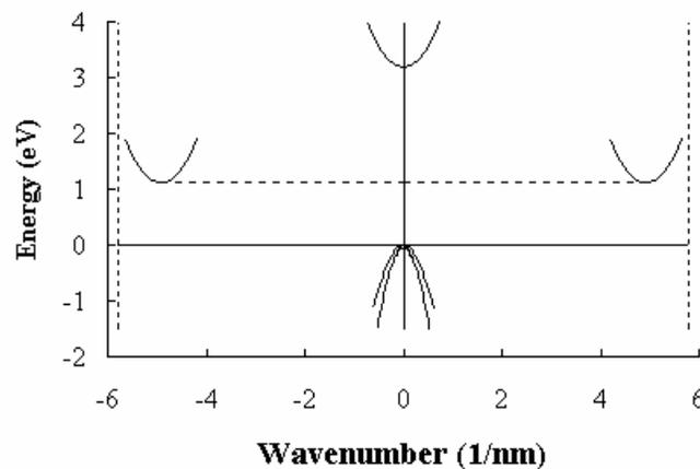
**Figure 2.3.12**  $E-k$  diagram of silicon including the primary band minima and maxima.
