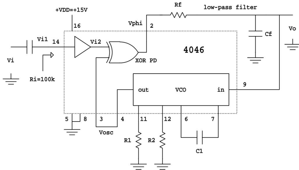
Figure 3: CMOS 4046 PLL: basic connection diagram.
