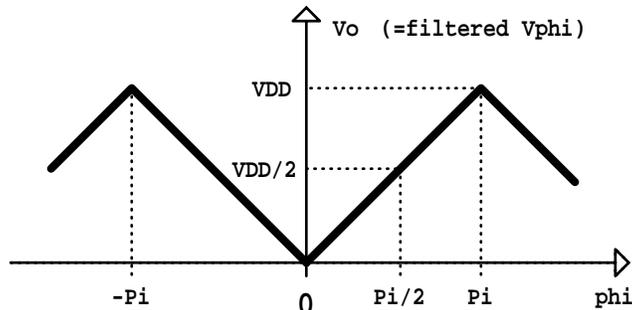
Figure 5: Characteristic of the phase detector.
