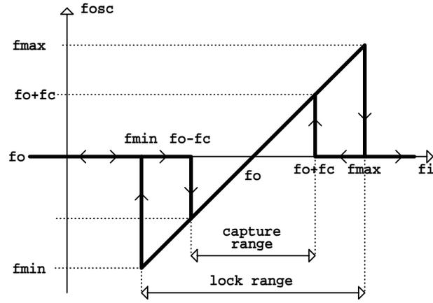
Figure 2: Steady-state  $f_{osc}(f_i)$  characteristic of the basic PLL.
