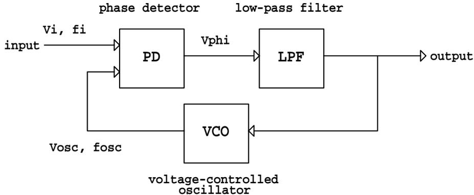
Figure 1: Block diagram of a basic phase-locked loop (PLL).
