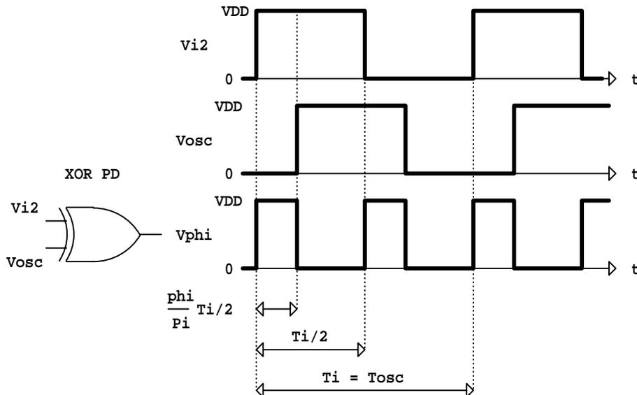
Figure 4: Operation of the phase detector with XOR gate.
