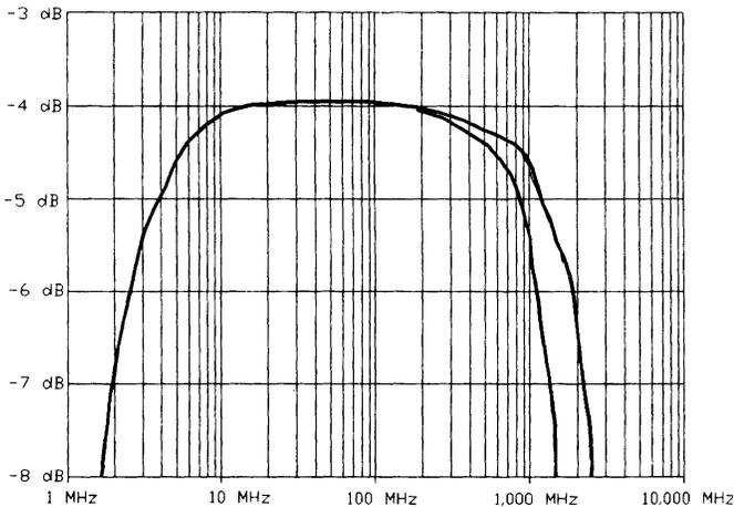
Figure 7: Insertion Loss Cure of a 4:1 Flux Coupled Transformer.
