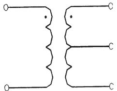
Figure 1. Flux Coupled Balun Transformer
