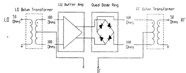
Figure 5. Double Balanced Mixer Using Two 4:1 Flux Coupled Balun Transformers
