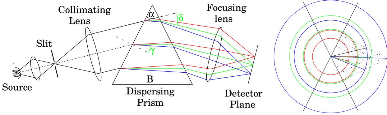
Figure 1: A simple prism spectroscope. The source is imaged onto a narrow slit and the emerging light is collimated by a lens. The refracted beams, emerging at different angles are focused by a second lens to give separate monochromatic images of the slit.
