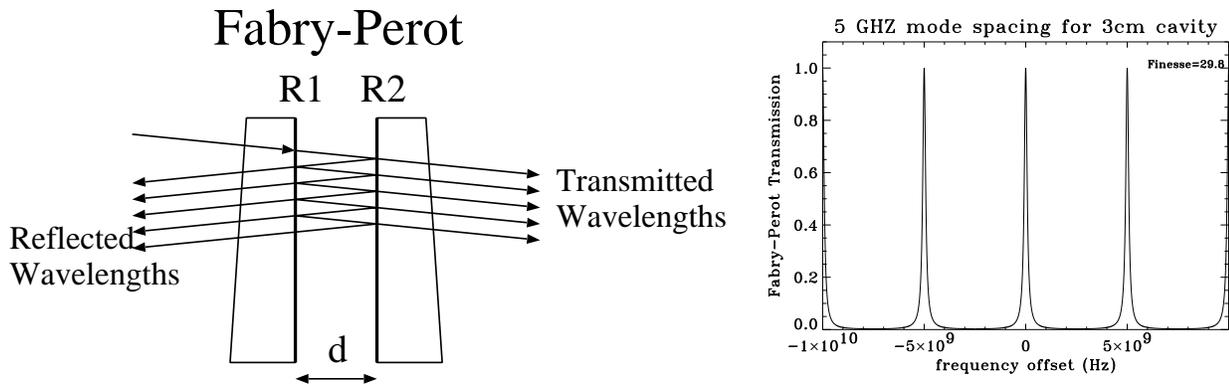
Figure 4: Fabry-Perot filter. (a) Consists of resonant cavity made by two highly reflective mirrors M1 and M2 separated by a distance  $d$  and aligned parallel to each other. (b) Transmission of light through a Fabry-Perot filter. The transmission occurs at frequencies spaced  $c/2d$  apart.
