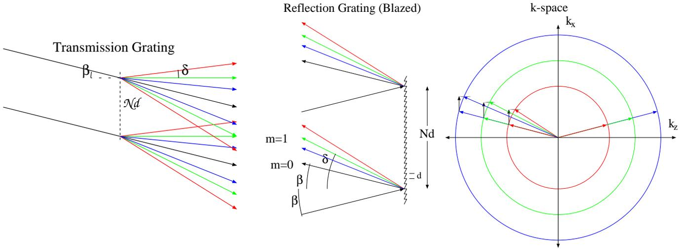
Figure 2: Geometry for determining the resolving power of a grating. The effective width of the grating is  $Nd \cos \delta_1$ , where the width of the grating is  $Nd$ . ( $N$ , the number of grating lines, and  $d$ , their separation.)
