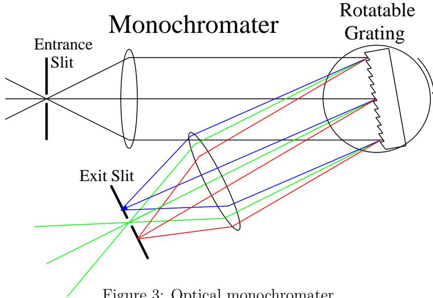
Figure 3: Optical monochromator
