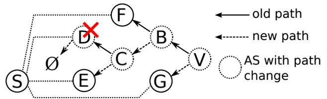
**Figure 2: General topology subgraph demonstrating a three-level induced path change starting at  $c$  and propagating up to  $v$  (impossible under the simplified routing model). The ASes shown can be anywhere in the path.**
